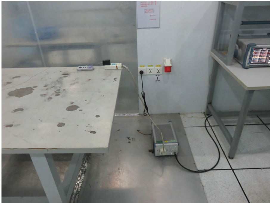
1 Photo of Power Line Conducted Emission Measurement
