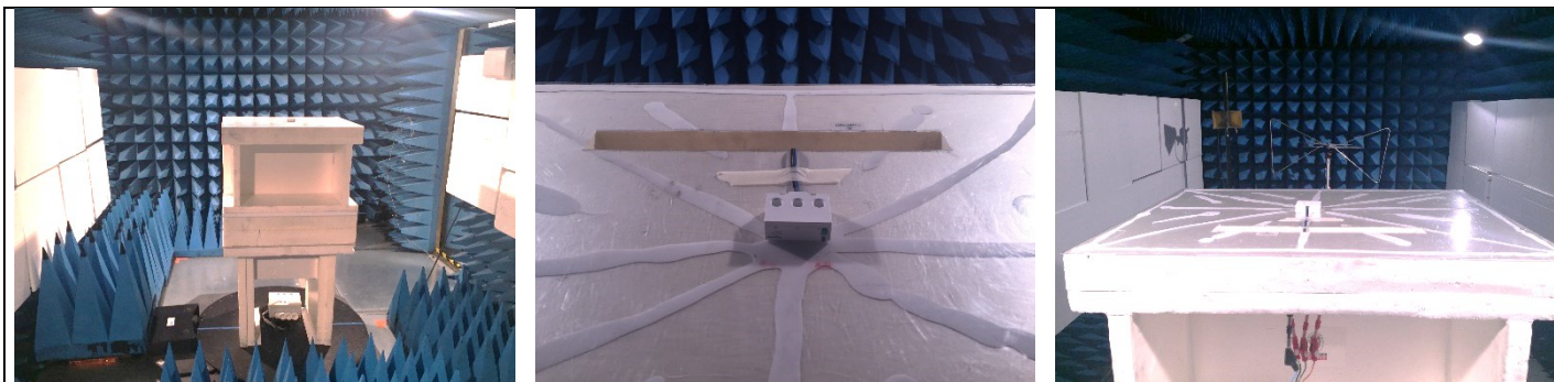
Test setup in anechoic chamber > 1GHz (Axis XY)
