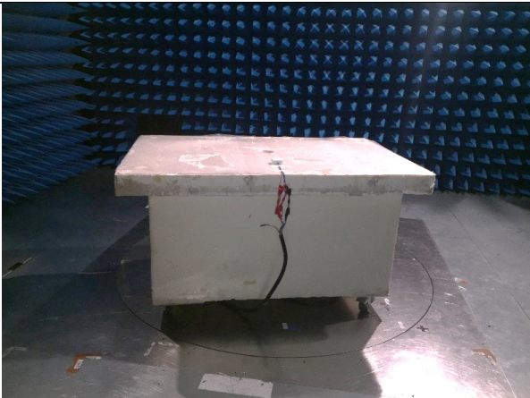
Test setup in anechoic chamber < 1GHz (Axis XY)
