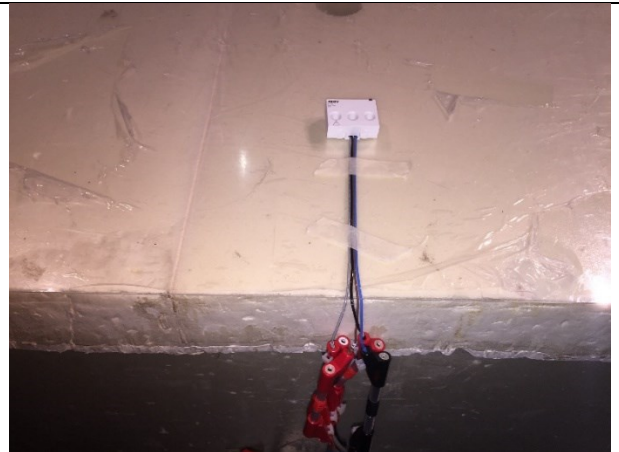
Test setup in anechoic chamber < 1GHz (Axis XY)
