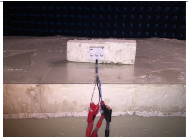
Test setup in anechoic chamber < 1GHz (Axis XY)
