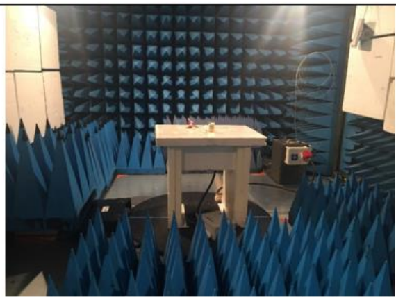
Test setup in anechoic chamber < 1GHz (Axis Z)
