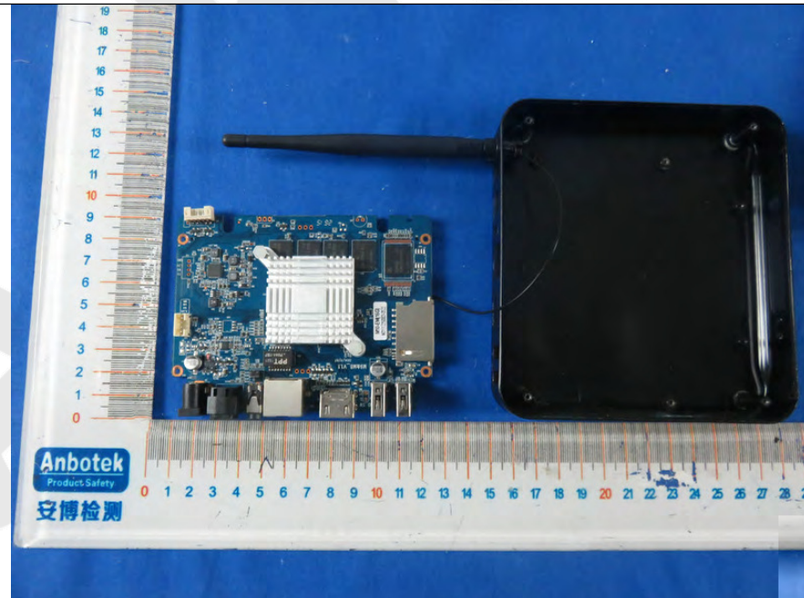
2. Figure The EUT-Antenna View
