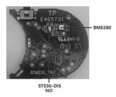
The BTM-250B no include an Environmental sensor that supports humidity and pressure along with temperature.
