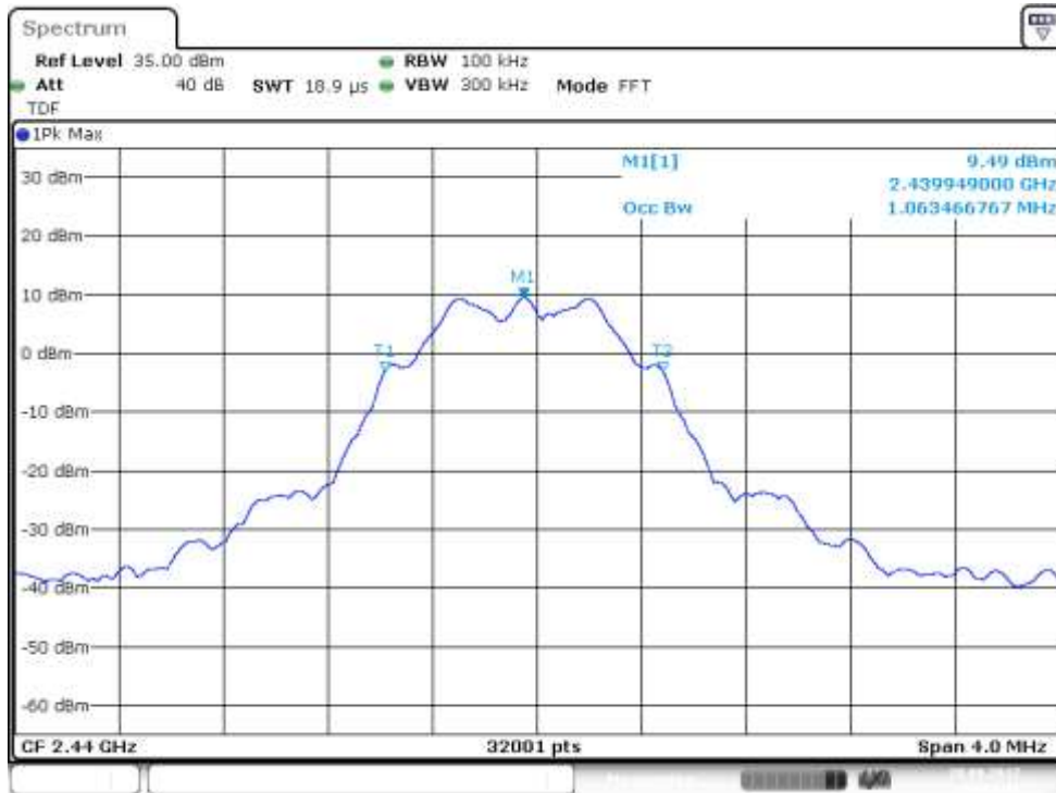
Figure 112: 99% OBW, Channel 19 mid (EUT 3), power setting 145
