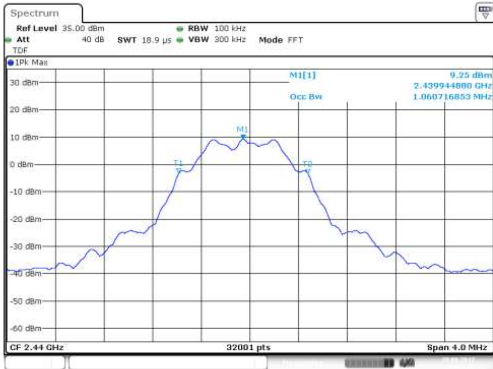
Figure 105: 99% OBW, Channel 19 mid (EUT 2), power setting 145
