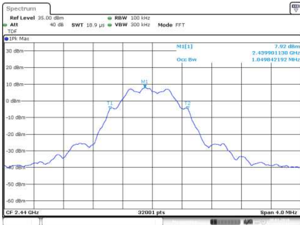
Figure 118: 99% OBW, Channel 0 low (EUT 4), power setting 104
