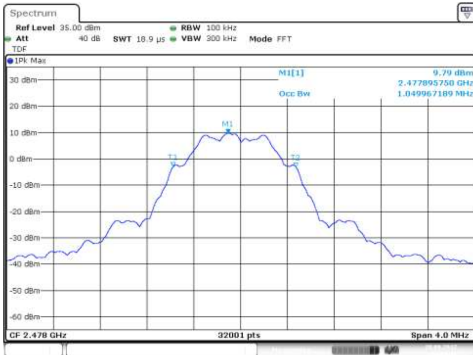
Figure 113: 99% OBW, Channel 38 high (EUT 3), power setting 145
