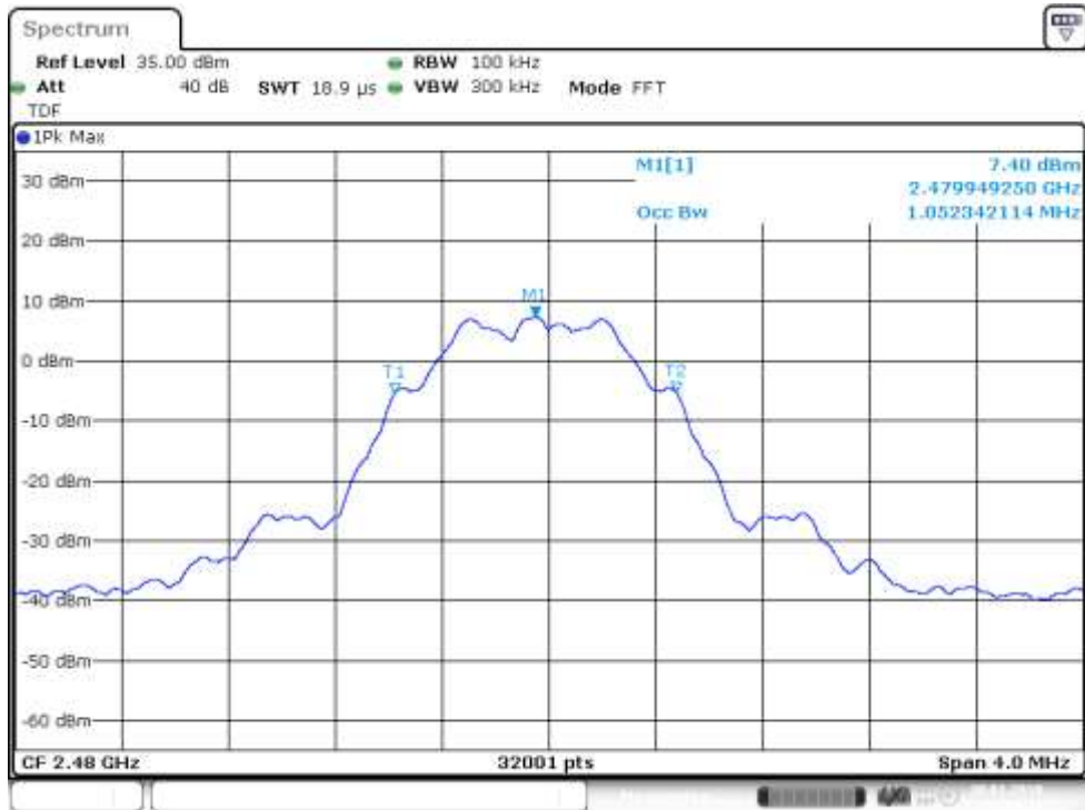
Figure 120: 99% OBW, Channel 39 high (EUT 4), power setting 104
