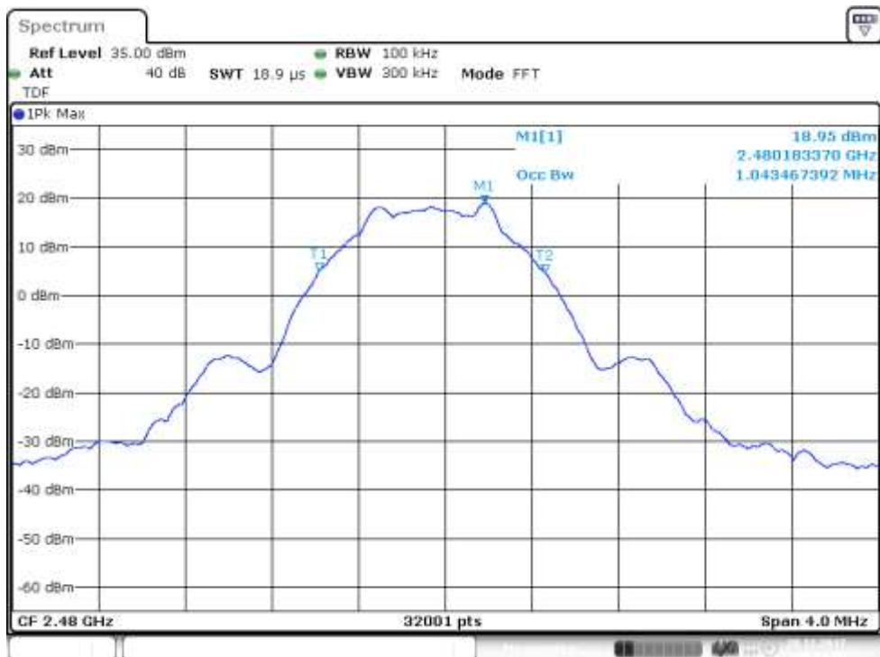
Figure 110: 99% OBW, Channel 39 high (EUT 2), power setting 200, PHY 1M coded
