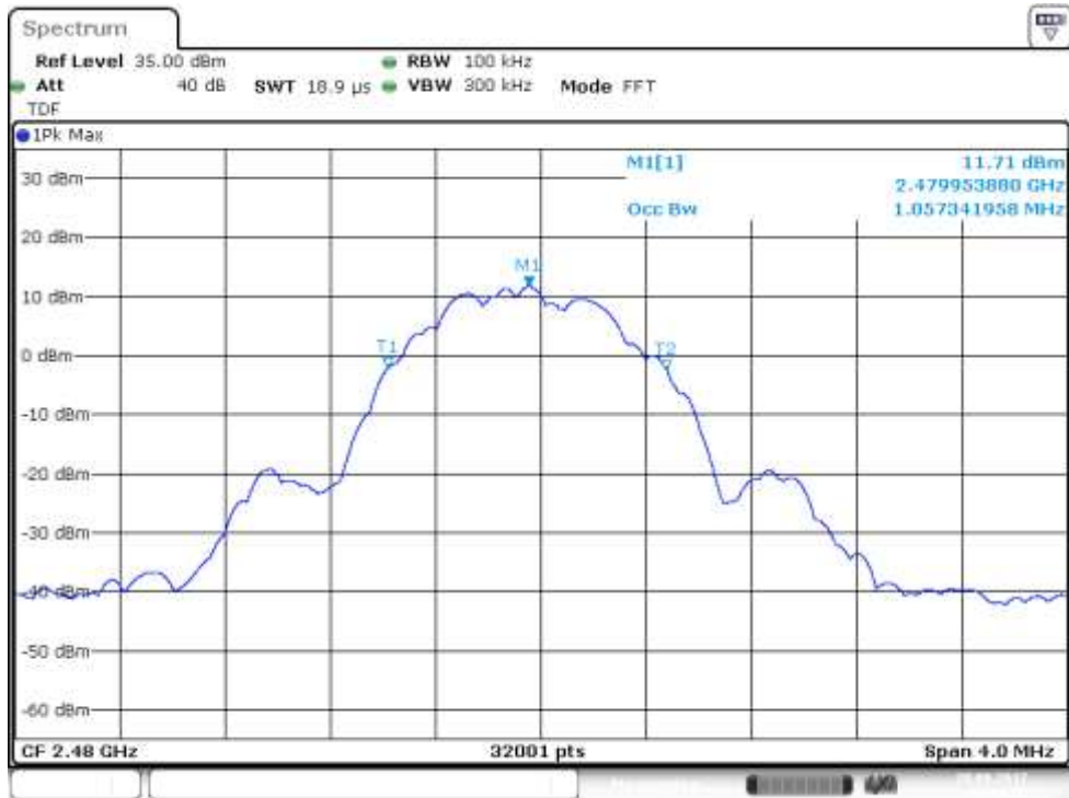
Figure 107: 99% OBW, Channel 39 high (EUT 2), power setting 145
