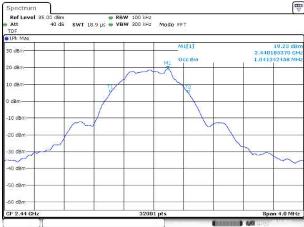
Figure 109: 99% OBW, Channel 19 mid (EUT 2), power setting 200, PHY 1M coded
