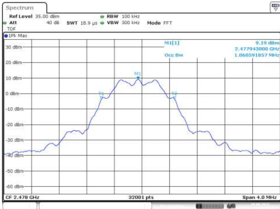
Figure 106: 99% OBW, Channel 38 high (EUT 2), power setting 145
