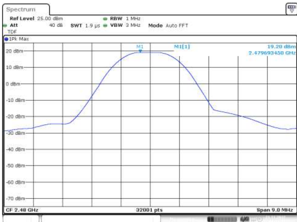
Figure 16: Conducted power, Channel 39 high (EUT 3), power setting 200, PHY 1M coded
