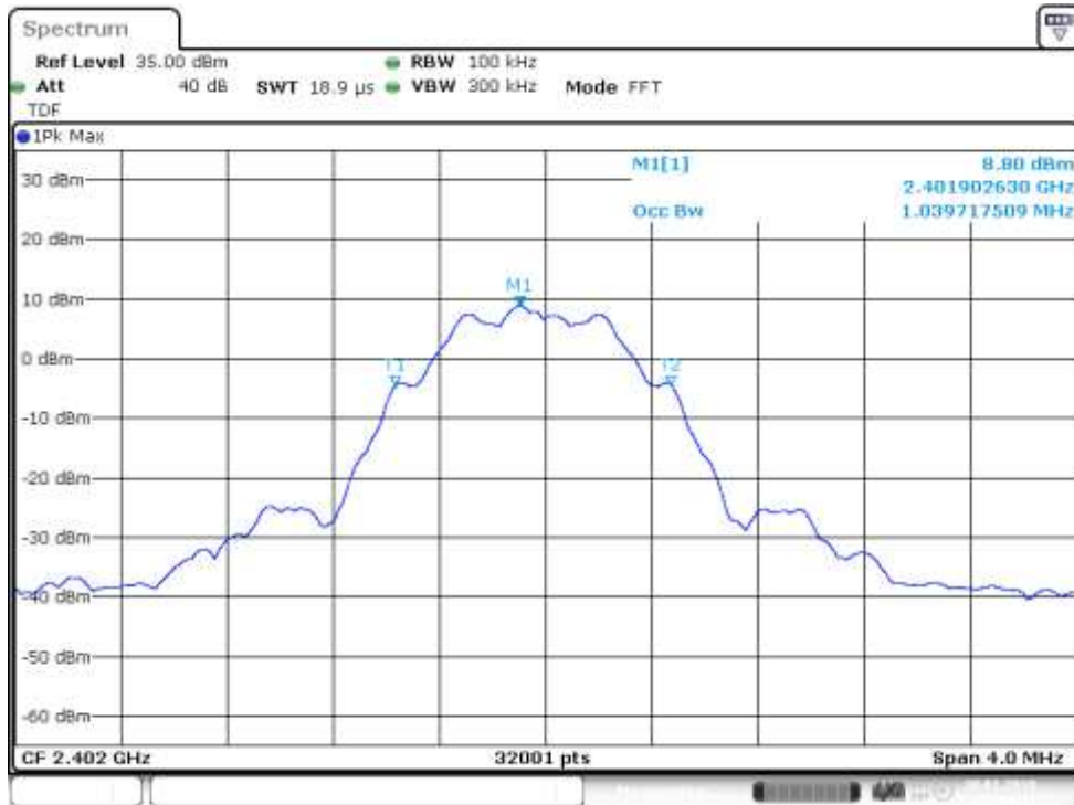
Figure 118: 99% OBW, Channel 0 low (EUT 4), power setting 104
