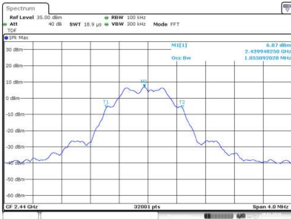
Figure 121: 99% OBW, Channel 0 low (EUT 5), power setting 104
