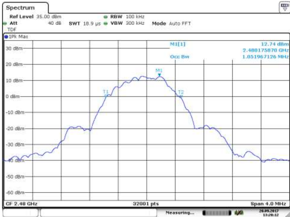
Figure 114: 99% OBW, Channel 39 high (EUT 3), power setting 145
