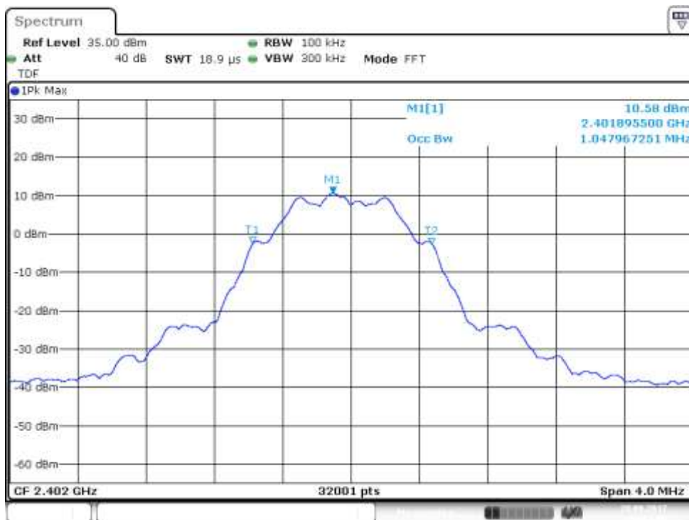
Figure 104: 99% OBW, Channel 0 low (EUT 2), power setting 145
