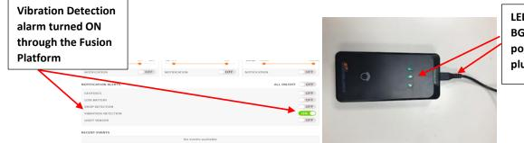
LEDs flashing and BG96 on when a powered USB is plugged into the BAT
