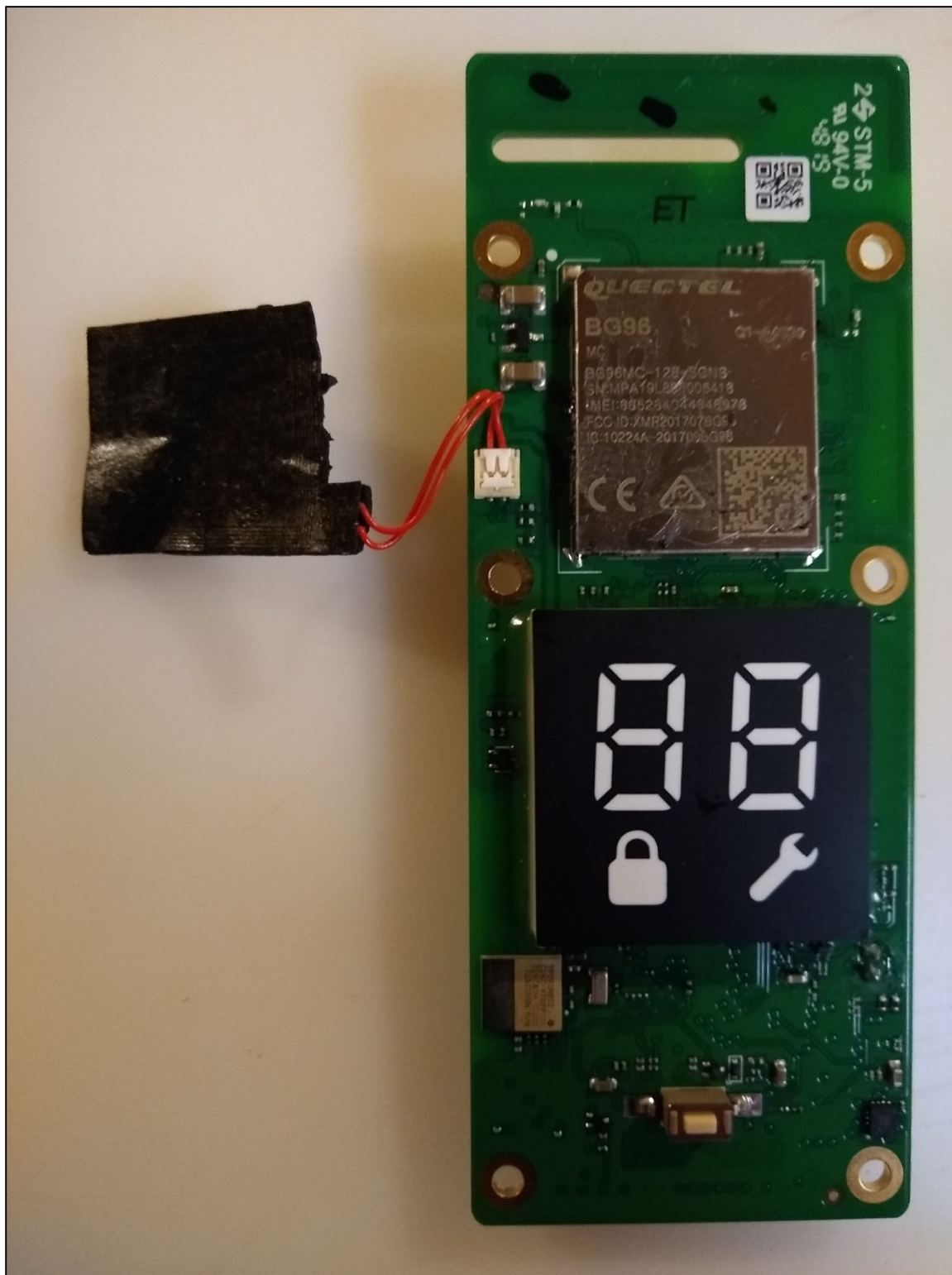
Photograph 4. PCB – Heat sensor removed to show Quectel BG96-MC module.
