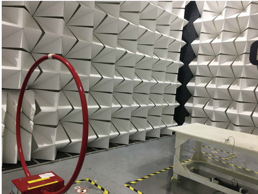
Radiated spurious emission Test Setup-1(Below 30MHz)
