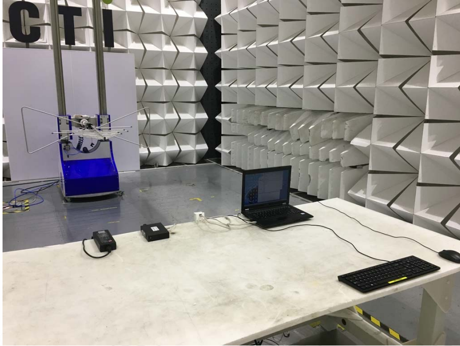
Radiated emission Test Setup-1(30MHz-1GHz)
