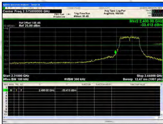
Out Of Band Emission IEEE 802.11g_Channel 1_20MHz_Antenna 1
