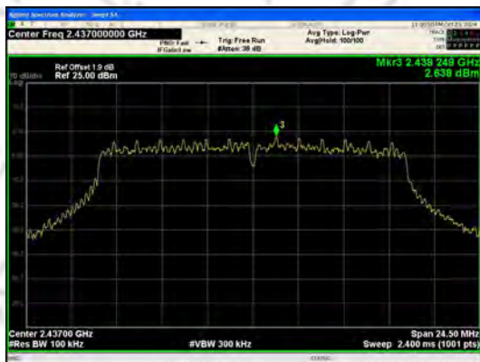
In-Band Reference Level IEEE 802.11g_Channel 6_20MHz_Antenna 0
