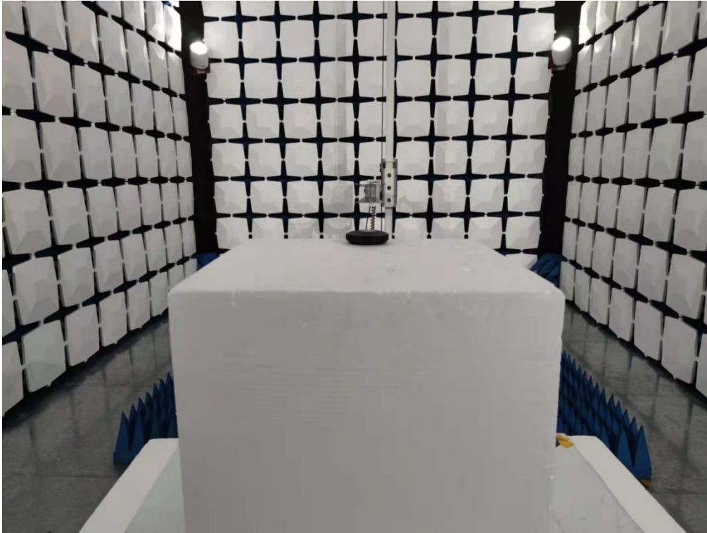
Above 1GHz for radiated emission test setup
