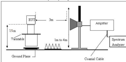
Radiated Emission Test-Up Frequency Above 1GHz
