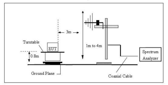
(C) Radiated Emission Test-Up Frequency Above 1GHz
