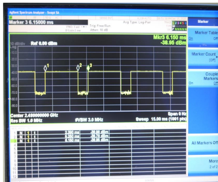
Time-domain plot for Bluetooth transmission signal
