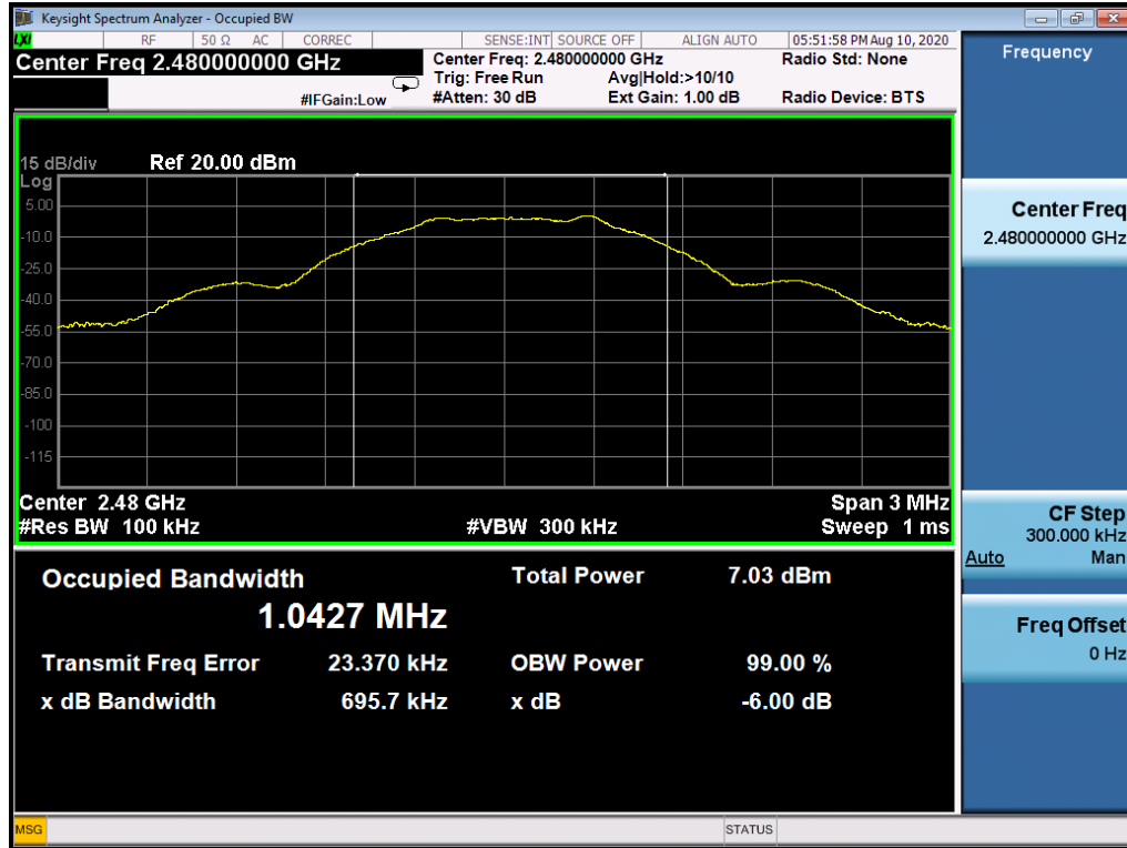
Figure 3: 6dB Bandwidth, 2480MHz
