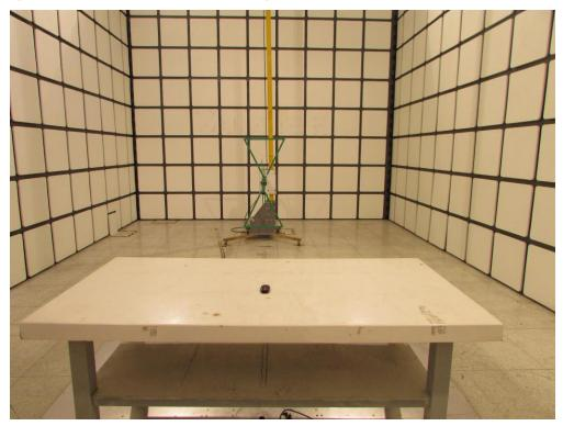
Description: Radiated Emission Test Setup for  $1\sim18GHz$
