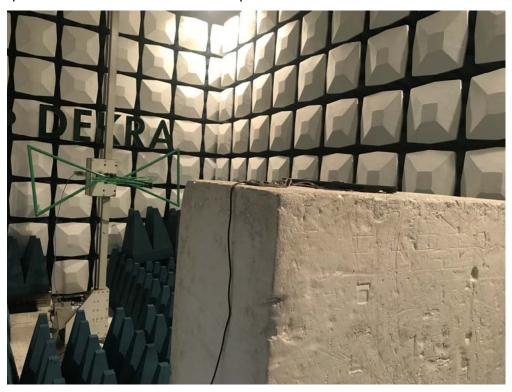
Description: Radiated Emission Test Setup for 1~18GHz
