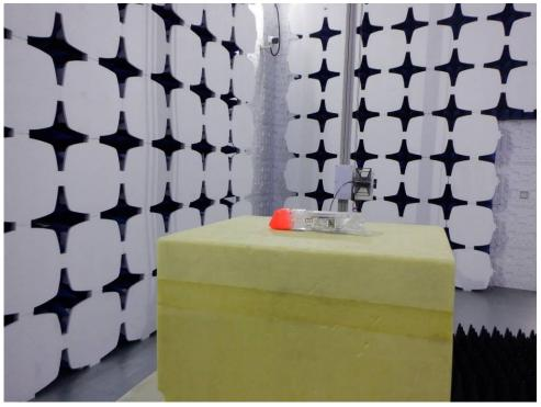
Radiated Spurious Emissions 9KHz-30MHz
