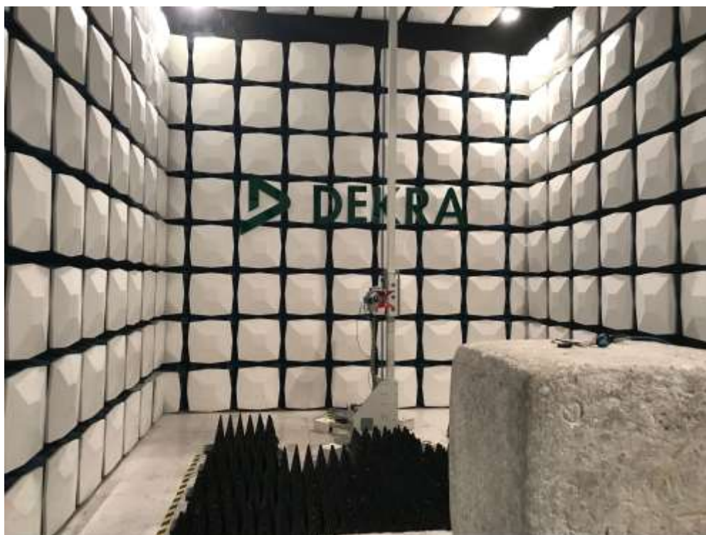
Description: Radiated Emission Test Setup for 1~18GHz
