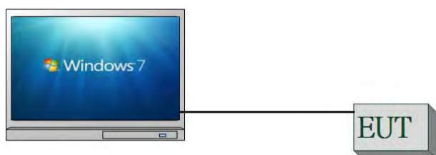
Fig. 2-1 Conducted (Antenna Port) Emission Configuration
