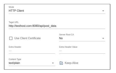
Users can simply use https:// in URL to enable HTTPS. And users can also enable Server Root CA/User Client Certificate based on the server requirement. The certificate files can be uploaded on the Security page.
