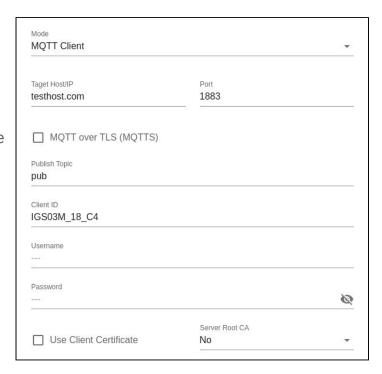
Users can enable MQTTS support. And also can enable Server Root CA/Use Client Certificate based on the server requirement. For example, to enable AWS-IOT, the user has to enable MQTTS/ROOT CA/ Use Certificate options and upload certificate and private key in the security page.
