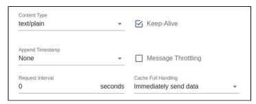
clients. The device will use HTTP persistent connection to reuse existing tcp sessions. This enhances the HTTP efficiency.
