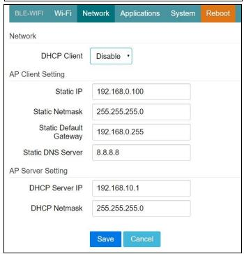
This setting is for AP mode. The default IP address of iGS01S in AP mode is 192.168.10.1 and the netmask is 255.255.255.0. In case the user want to change the IP address in AP mode, just set the IP and Netmask here. The corresponding DHCP client address will be changed too. For example, if the DHCP server IP address is changed to 192.168.0.1, the DHCP clients associated to iGS01S AP will be 192.168.0.X.
