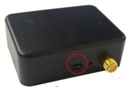
It is used to act WPS, reset to default settings, and OTA (over-the-air FW upgrade). Below is how it functions.
