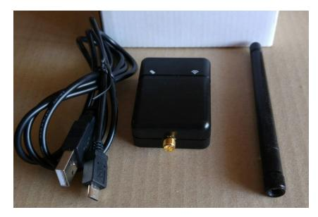
Inside the Box, there are one iGS01 unit, one 1M USB cable, and one 2dBi dipole antenna. iGS01 is powered by a standard micro-USB cable, rated at 5V&500mA. You can power this device with a standard smartphone charger or the USB port of any host device that can support 500mA or above.
