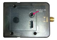
It is used to act WPS, reset to default settings, and OTA (over-the-air FW upgrade). Below is how it
