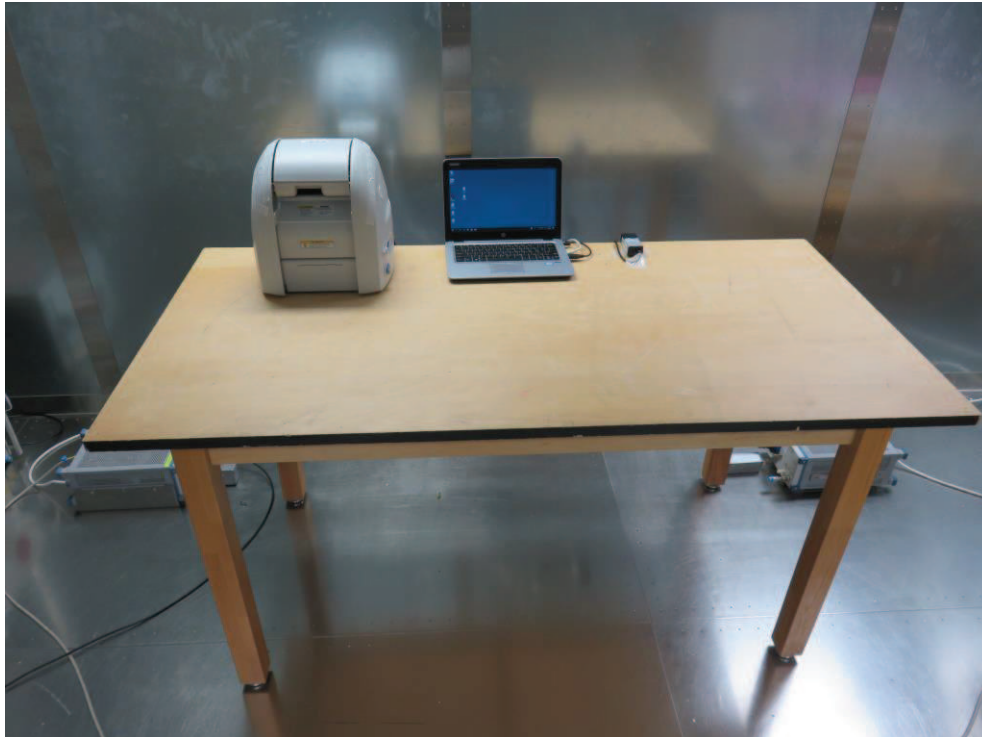
Photograph 3: Set-up for AC Power Line Conducted Emission of Transmitter, Front View
