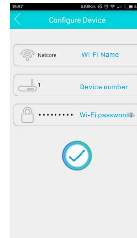
⑤ Lamp Status from red - green - blue cycling flashes green until white long bright, that means successful configuration. Then the APP will automatically search for the device with the current successful configuration.
