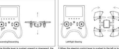
When the throttle lever is pushed upward or downward, the Quad-rotor will fly to upward or downward. 2. When the steering control lever is pushed to the left or to the right, the head of the Quad-rotor will rotate to the left or to the
