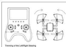
5.Adjust the Steering Trimmer, if the head of the Quad-rotor deviates to the left when taking off, please trim it to the right.
