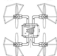
3. When taking picture, press the Camera key, the green indicator on the Camera Board will be OFF and the red indicator will be flashing for a while and then the green indicator will keep eternal bright "ON" (press it one time for one piece).
