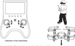
The Steering Control of the Quad-rotor under the Non-head Mode
