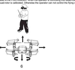
(1)When pushing the control lever of the transmitter forward, the Quad-rotor will fly toward the front direction following the standard direction of the Quad-rotor when it is calibrated.
