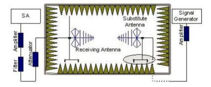
In the chamber, an substitution antenna for the frequency band of interest is placed at the reference point of the chamber. An RF Signal source for the frequency band of interest is connected to the substitution antenna with a cable that has been constructed to not interfere with the radiation pattern of the antenna. A
