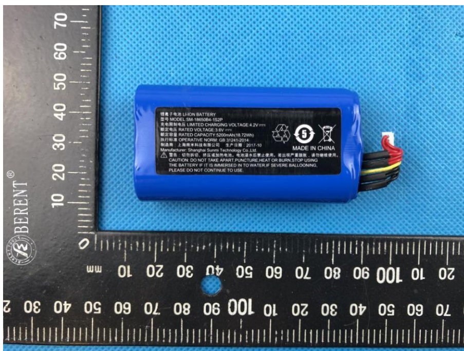
Picture13 : Photo of Battery (BA04)
