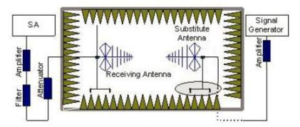
In the chamber, an substitution antenna for the frequency band of interest is placed at thereference point of the chamber. An RF Signal source for the frequency band of interest isconnected to the substitution antenna with a cable that has been constructed to not interferewith the radiation pattern of the antenna. A power (P<sub>Mea</sub>) is applied to the input of thesubstitution
