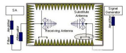
In the chamber, an substitution antenna for the frequency band of interest is placed at thereference point of the chamber. An RF Signal source for the frequency band of interest isconnected to the substitution antenna with a cable that has been constructed to not interfere with the radiation pattern of the antenna. A power (PMea) is applied to the input of the substitution
