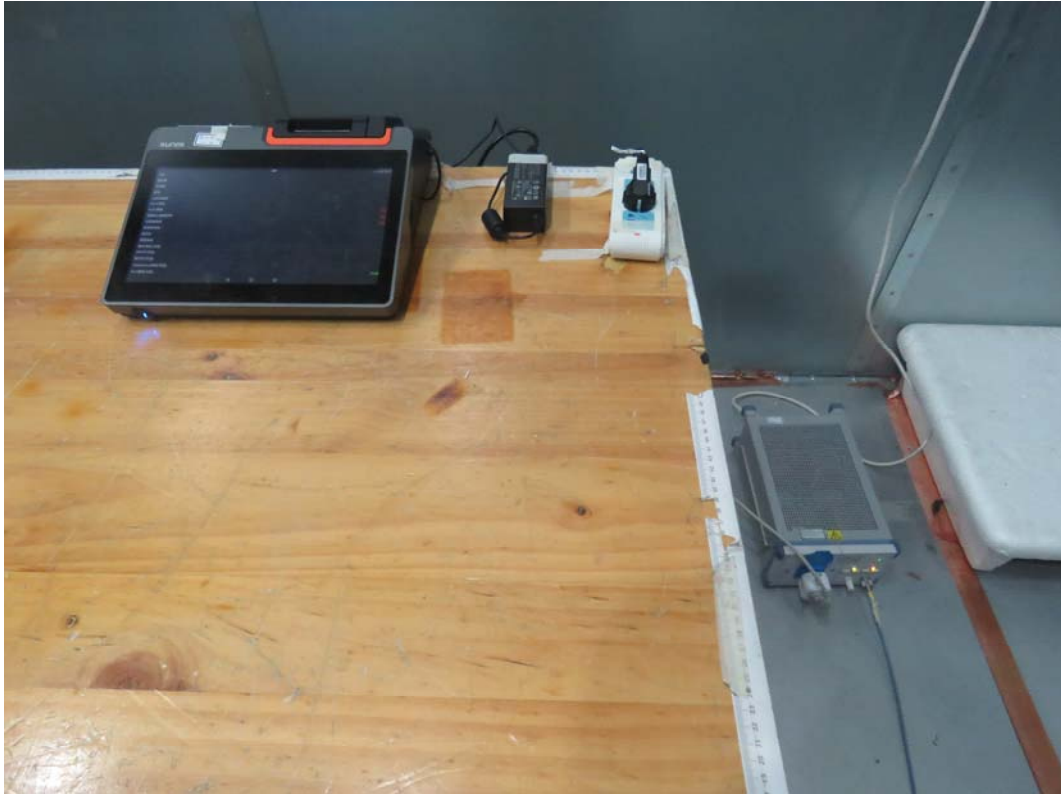
Picture 3 Conducted Emission Test Setup
