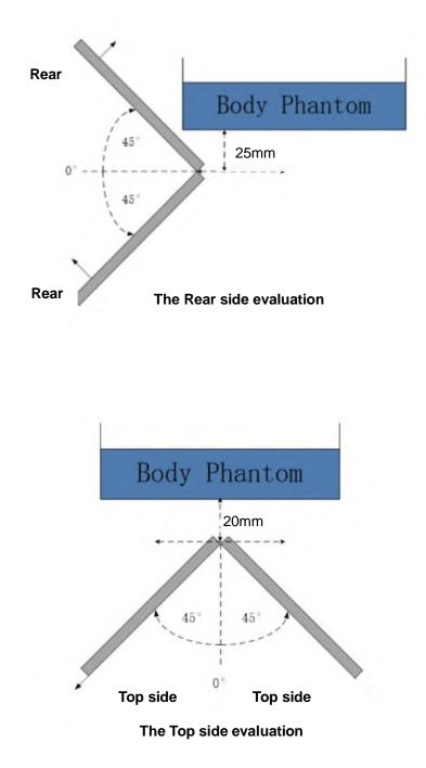
Based on the above evaluation, we come to the conclusion that the sensor triggering is not released and normal maximum output power is not restored within the  $\pm 45^{\circ}$  range at the smallest sensor triggering test distance declared by manufacturer.
