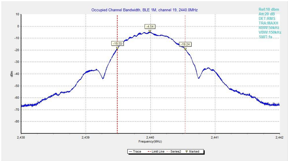
Fig.28 99% Occupied Bandwidth (Ch 19), LE 1M
