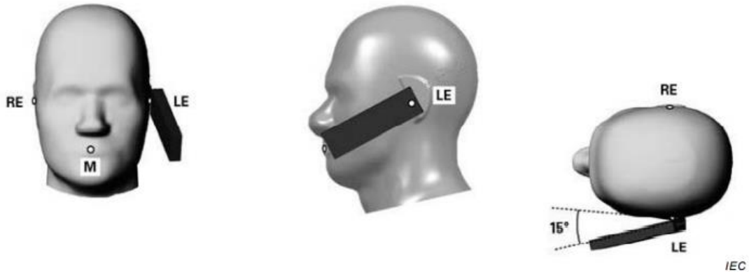
Picture 8-4 Tilt position of the wireless device on the left side of SAM
