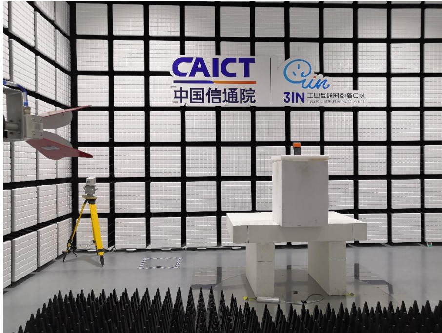
Description: Radiated Emission Test Setup (1GHz -18GHz)
