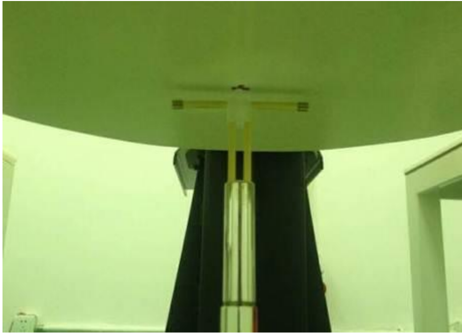
Picture 8.2 Photo of Dipole Setup
