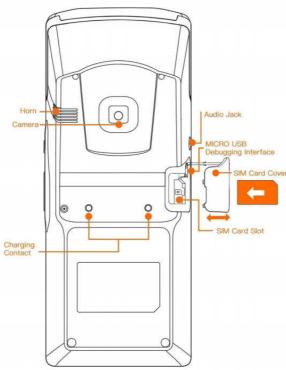
Inserting or removing card in power-on state may cause malfunction.
