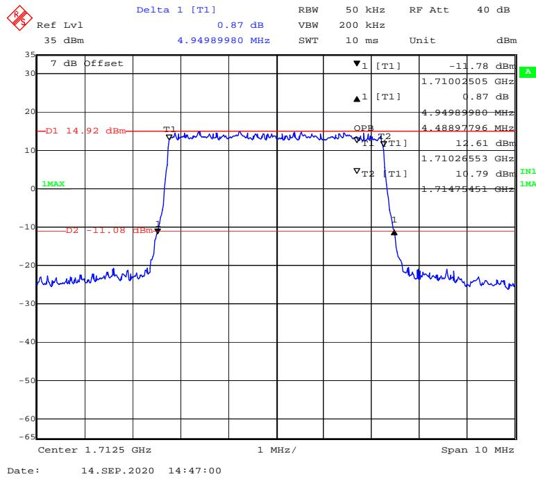
**16-QAM (10 MHz) - 99% Occupied & 26 dB Emissions Bandwidth, Low channel**
