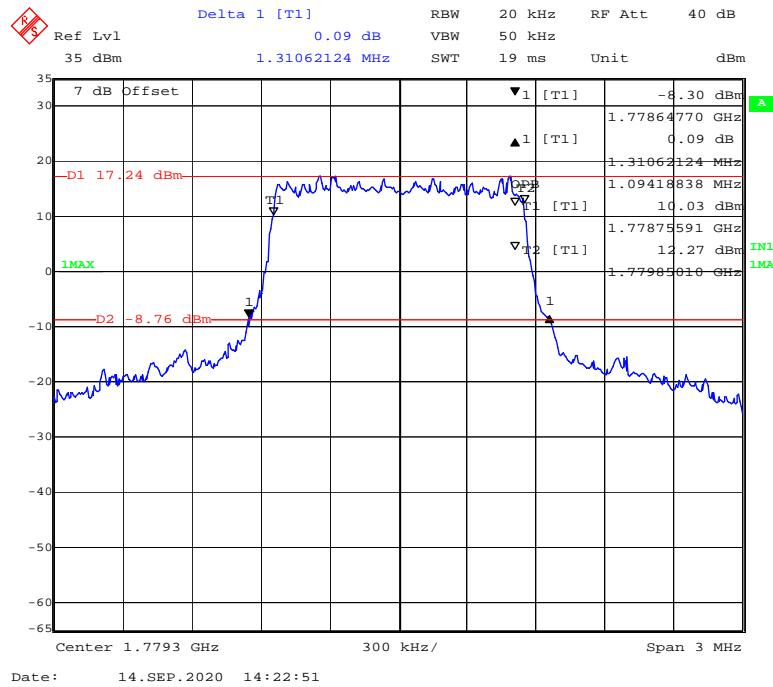
**16-QAM (3 MHz) - 99% Occupied & 26 dB Emissions Bandwidth, High channel**
