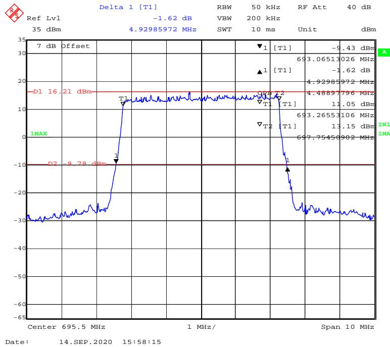
**QPSK (10MHz) - 99% Occupied & 26 dB Emissions Bandwidth, High channel**
