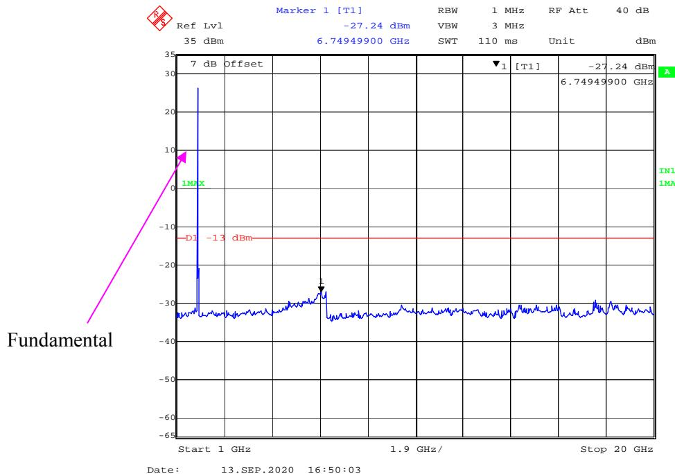
**30 MHz – 1GHz WCDMA (HSPA+) Mode, Low channel**
