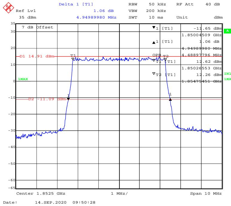
**16-QAM (10 MHz) - 99% Occupied & 26 dB Emissions Bandwidth, Low channel**
