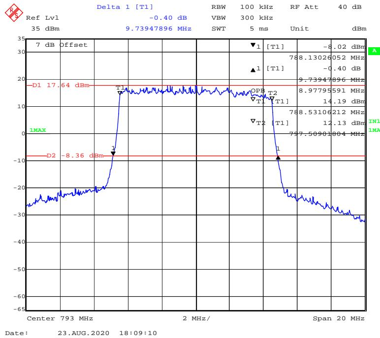
**QPSK (5 MHz) - 99% Occupied & 26 dB Emissions Bandwidth, High channel**
