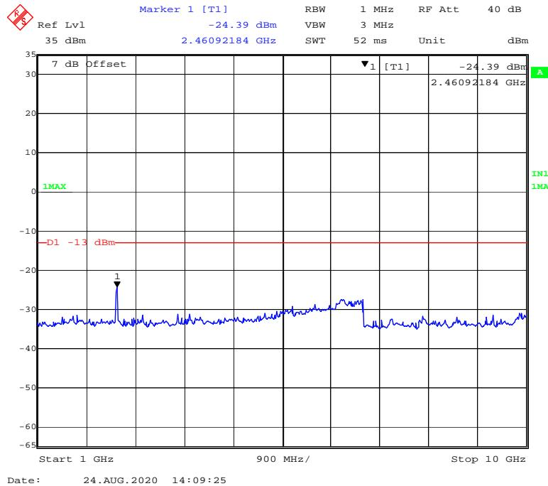
**30 MHz – 1GHz WCDMA (Rel 99) Mode, High channel**
