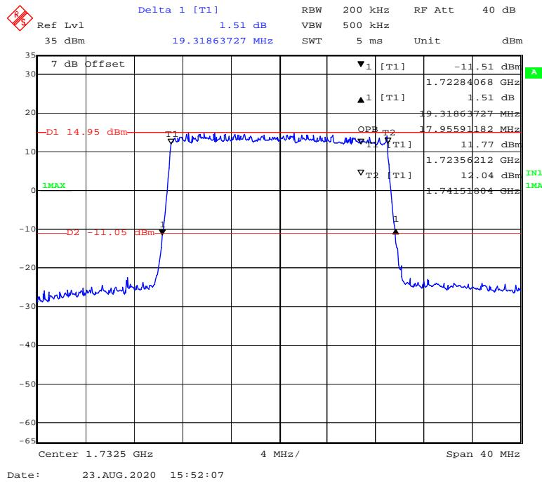
**16-QAM (1.4 MHz) - 99% Occupied & 26 dB Emissions Bandwidth, Middle channel**
