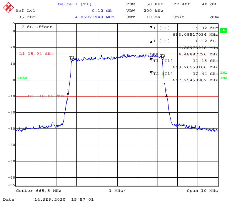
**16-QAM (10 MHz) - 99% Occupied & 26 dB Emissions Bandwidth, Low channel**
