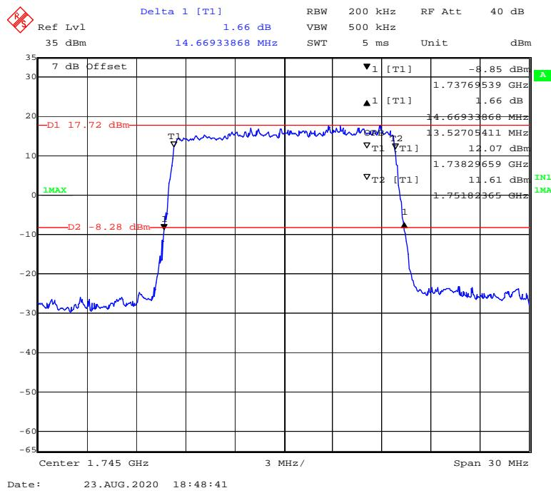
**QPSK (20 MHz) - 99% Occupied & 26 dB Emissions Bandwidth, Middle channel**
