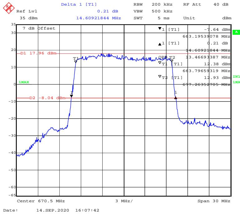
**16-QAM (20 MHz) - 99% Occupied & 26 dB Emissions Bandwidth, Low channel**
