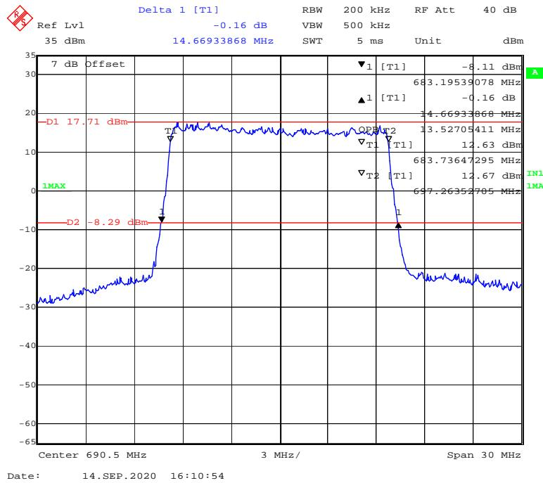
**16-QAM (20 MHz) - 99% Occupied & 26 dB Emissions Bandwidth, High channel**
