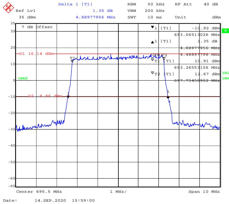
**16-QAM (10 MHz) - 99% Occupied & 26 dB Emissions Bandwidth, High channel**
