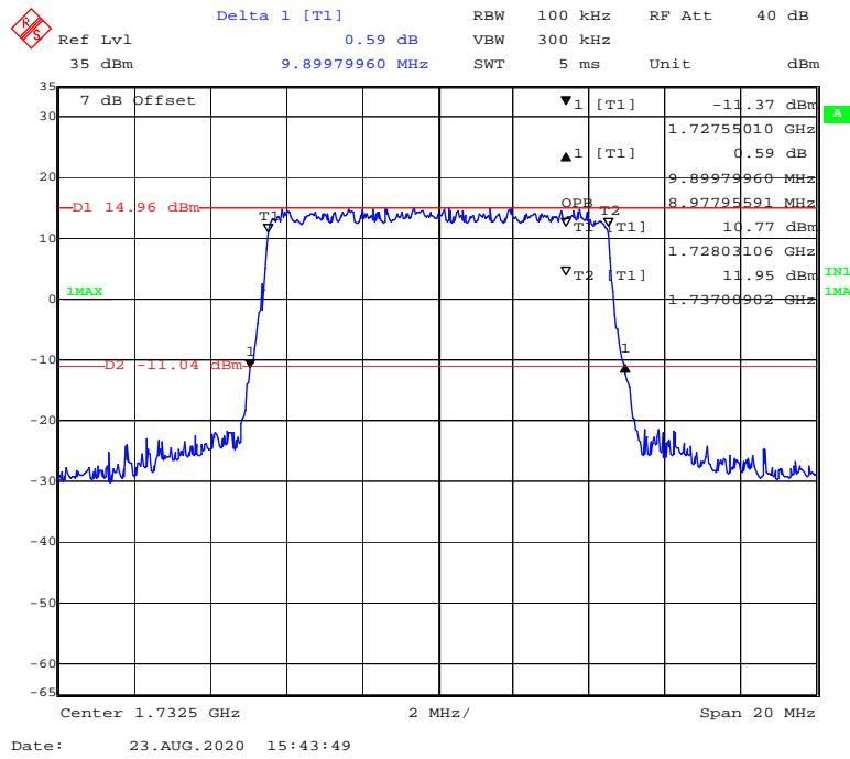
**QPSK (15 MHz) - 99% Occupied & 26 dB Emissions Bandwidth, Middle channel**
