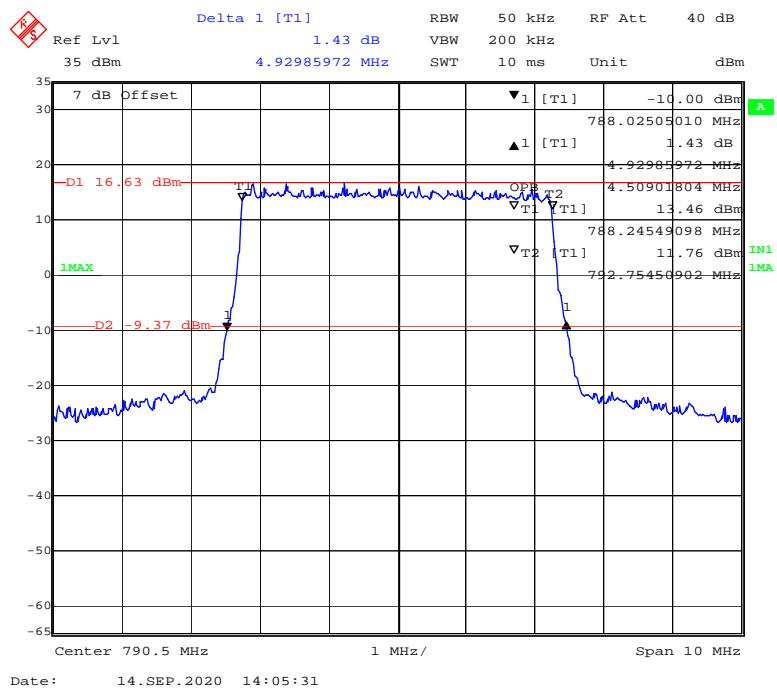
**QPSK (5 MHz) - 99% Occupied & 26 dB Emissions Bandwidth, Middle channel**
