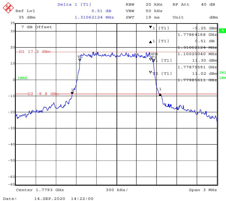
**QPSK (3 MHz) - 99% Occupied & 26 dB Emissions Bandwidth, High channel**
