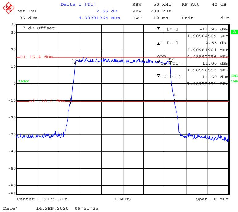
**QPSK (10MHz) - 99% Occupied & 26 dB Emissions Bandwidth, High channel**
