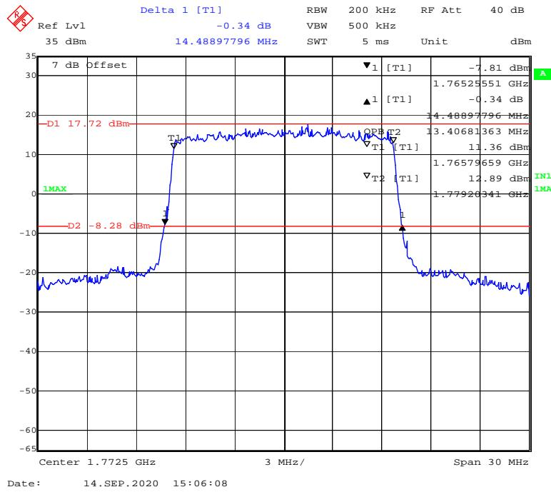
**QPSK (20 MHz) - 99% Occupied & 26 dB Emissions Bandwidth, High channel**
