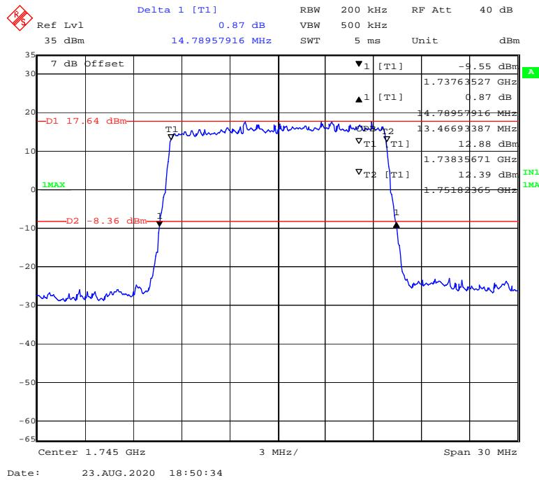
**16-QAM (20 MHz) - 99% Occupied & 26 dB Emissions Bandwidth, Middle channel**
