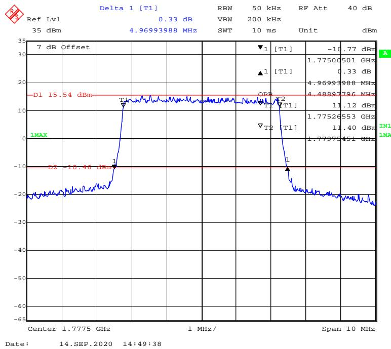
**16-QAM (10 MHz) - 99% Occupied & 26 dB Emissions Bandwidth, High channel**
