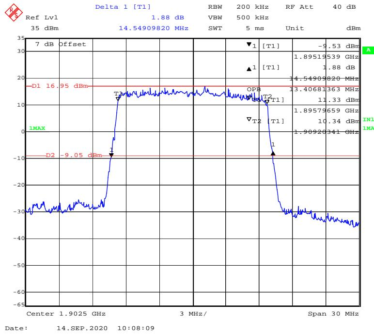
**QPSK (20 MHz) - 99% Occupied & 26 dB Emissions Bandwidth, High channel**
