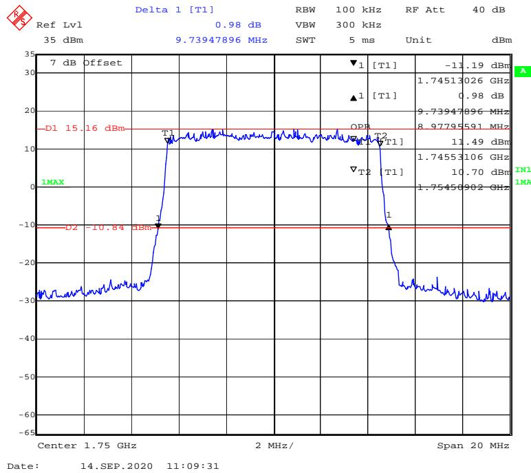
**QPSK (15 MHz) - 99% Occupied & 26 dB Emissions Bandwidth, High channel**
