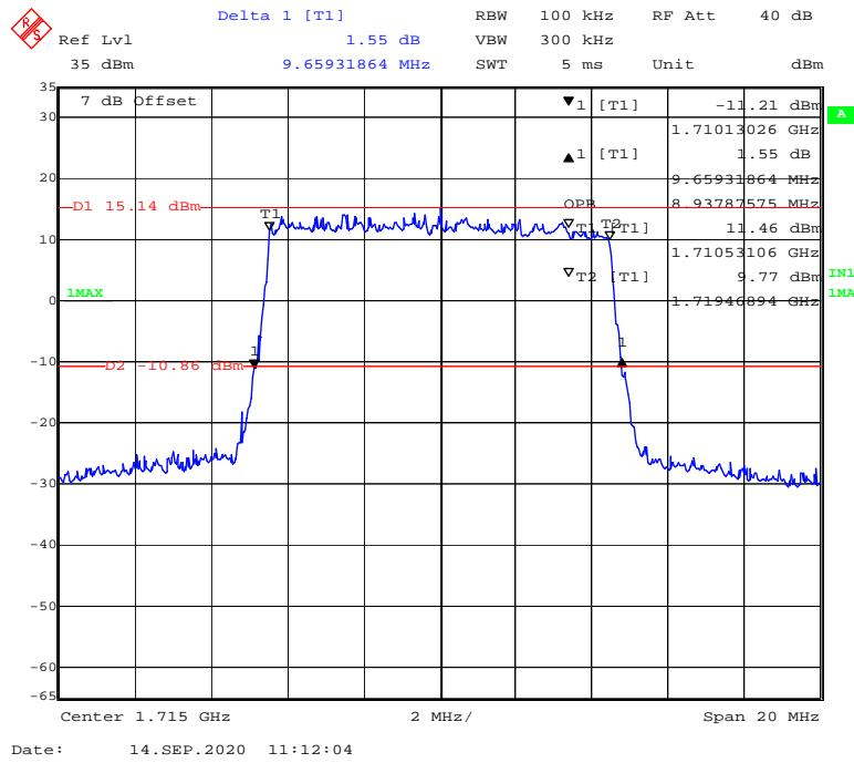
**QPSK (15 MHz) - 99% Occupied & 26 dB Emissions Bandwidth, Low channel**
