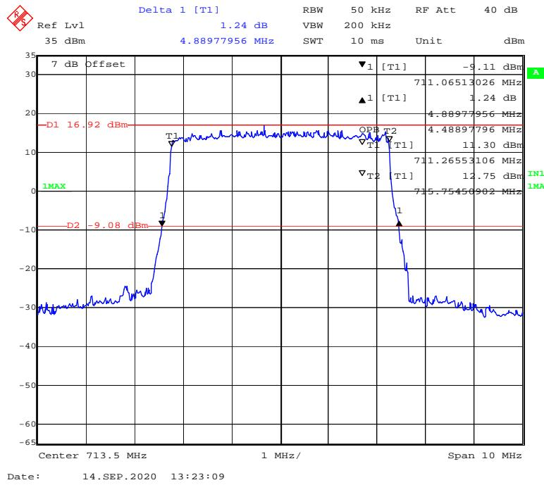
**16-QAM (10 MHz) - 99% Occupied & 26 dB Emissions Bandwidth, High channel**
