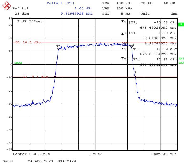
**16-QAM (15 MHz) - 99% Occupied & 26 dB Emissions Bandwidth, Middle channel**
