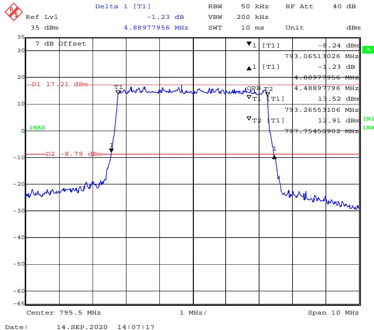
**16-QAM (5MHz) - 99% Occupied & 26 dB Emissions Bandwidth, High channel**
