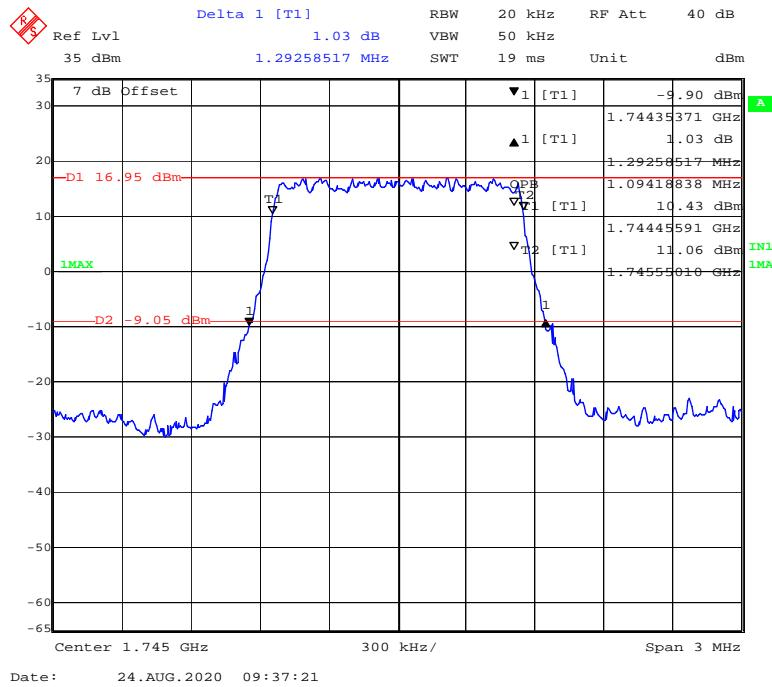
**16-QAM (3 MHz) - 99% Occupied & 26 dB Emissions Bandwidth, Middle channel**
