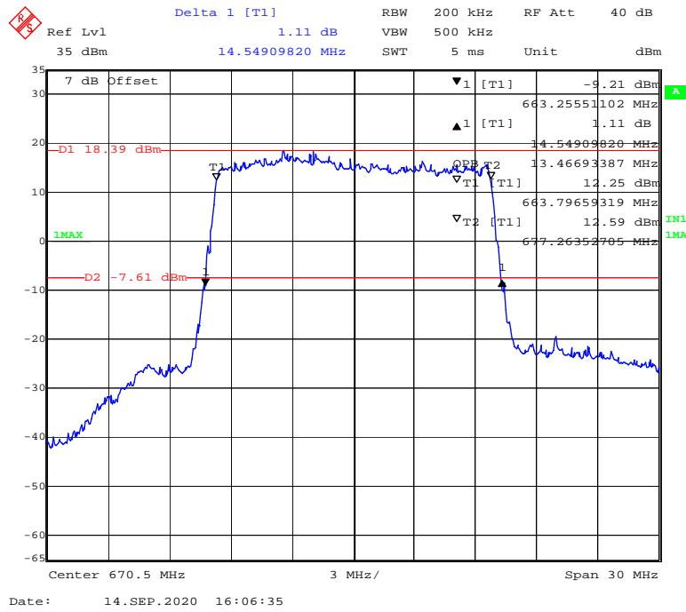
**QPSK (20 MHz) - 99% Occupied & 26 dB Emissions Bandwidth, Low channel**
