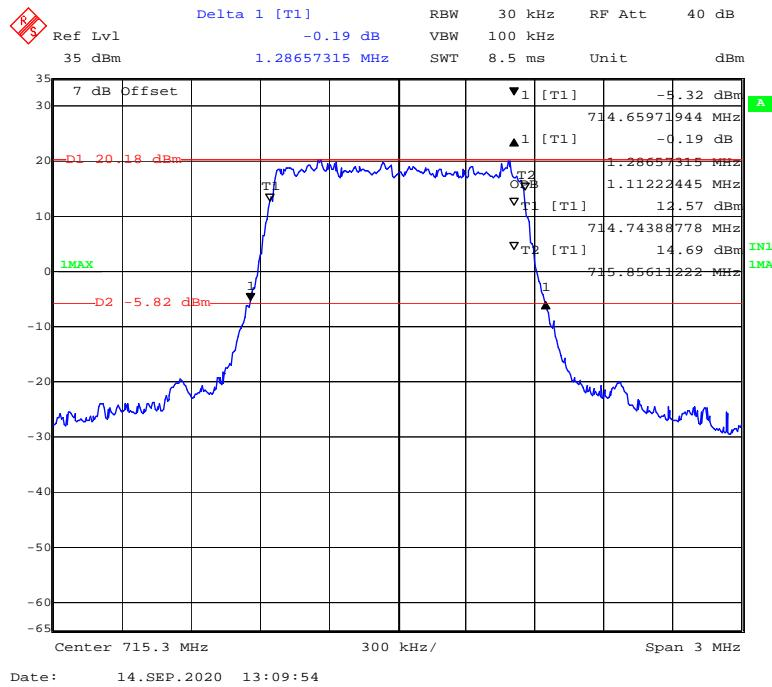
**16-QAM (3 MHz) - 99% Occupied & 26 dB Emissions Bandwidth, High channel**
