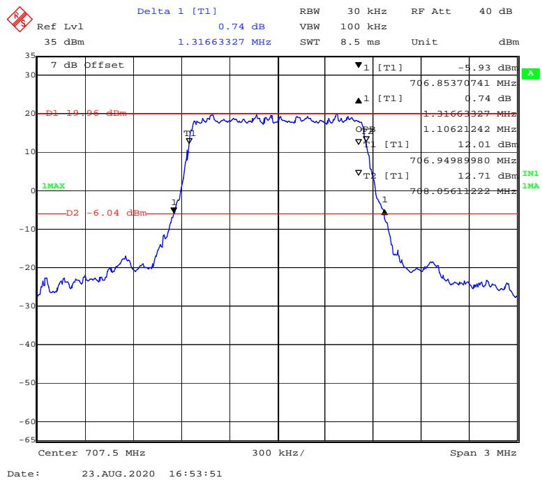
**QPSK (3 MHz) - 99% Occupied & 26 dB Emissions Bandwidth, Middle channel**
