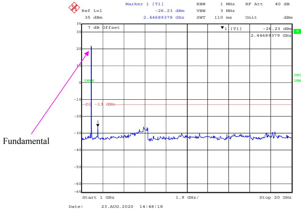
**30 MHz - 1 GHz (20 MHz, QPSK, Middle Channel)**
