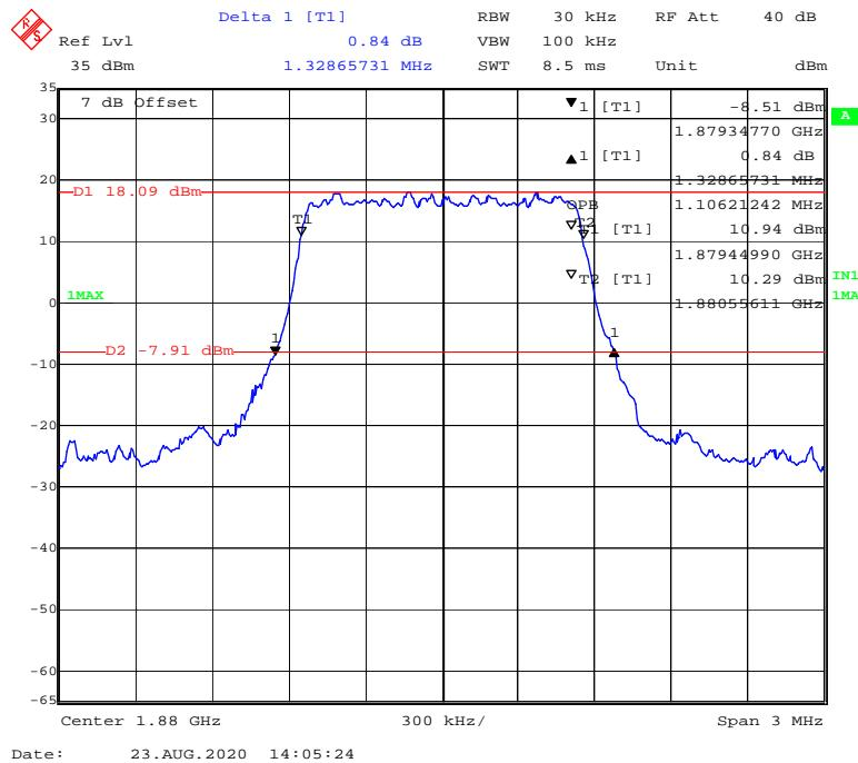
**QPSK (3 MHz) - 99% Occupied & 26 dB Emissions Bandwidth, Middle channel**
