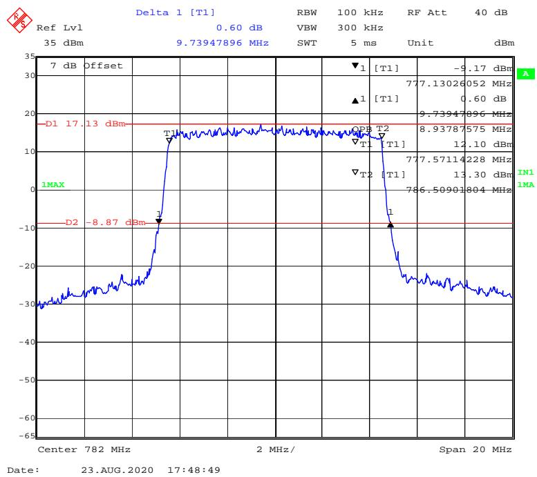
**16-QAM (5MHz) - 99% Occupied & 26 dB Emissions Bandwidth, Middle channel**
