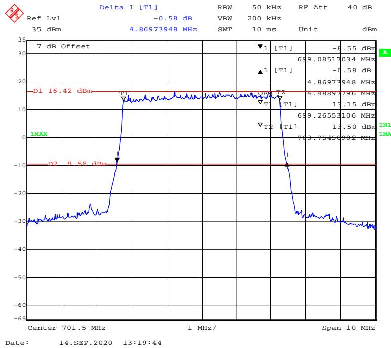
**QPSK (10MHz) - 99% Occupied & 26 dB Emissions Bandwidth, Low channel**
