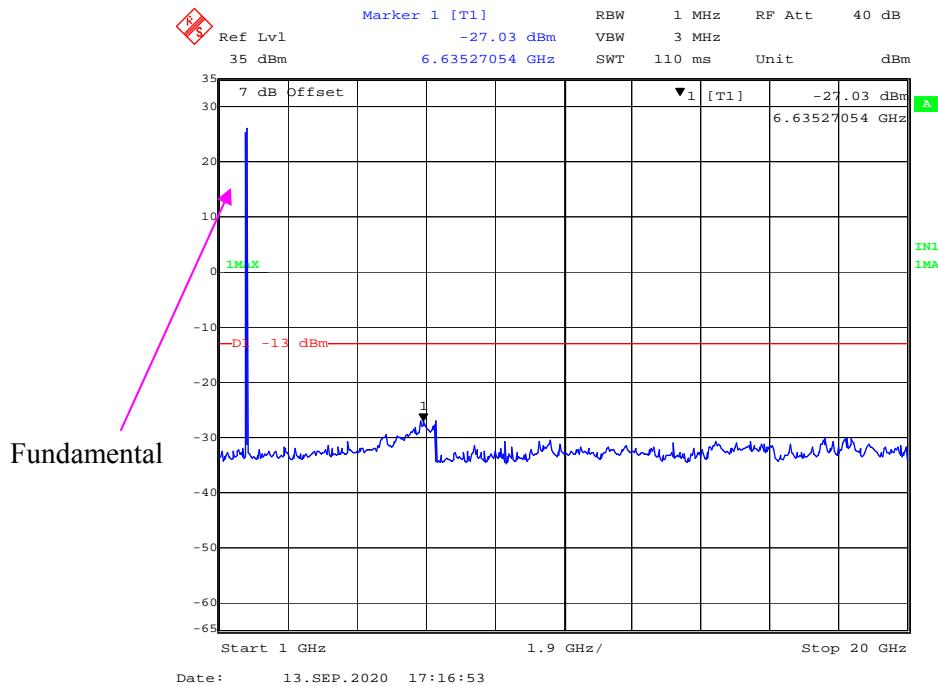
**30 MHz – 1GHz WCDMA (HSPA+) Mode, High channel**
