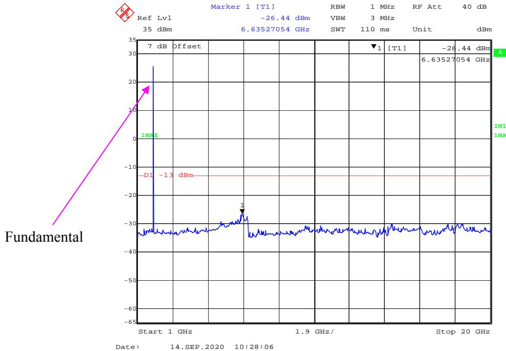
**30 MHz - 1 GHz (3 MHz, QPSK, Low Channel)**
