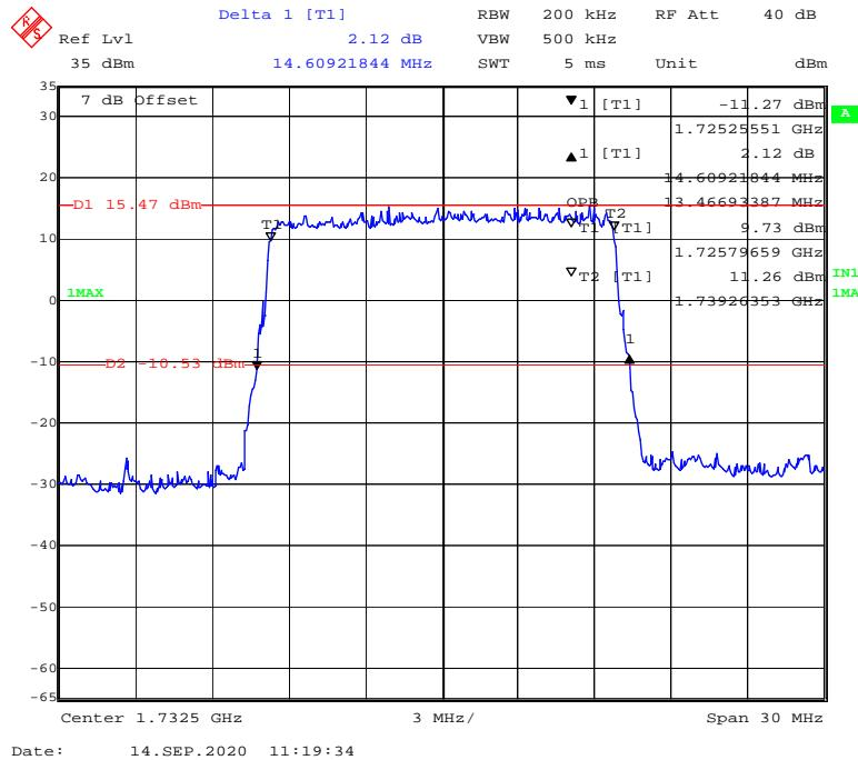
**16-QAM (20 MHz) - 99% Occupied & 26 dB Emissions Bandwidth, Middle channel**
