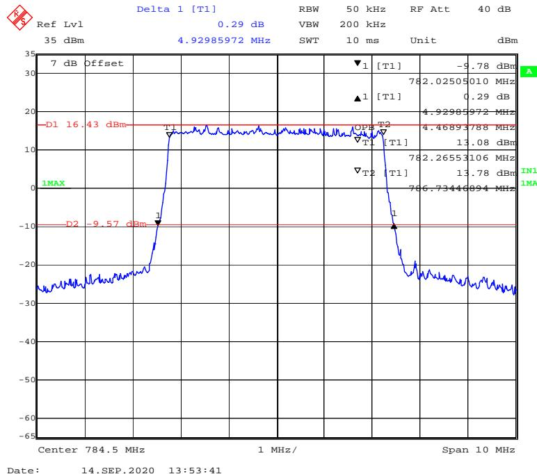
**16-QAM (5MHz) - 99% Occupied & 26 dB Emissions Bandwidth, High channel**
