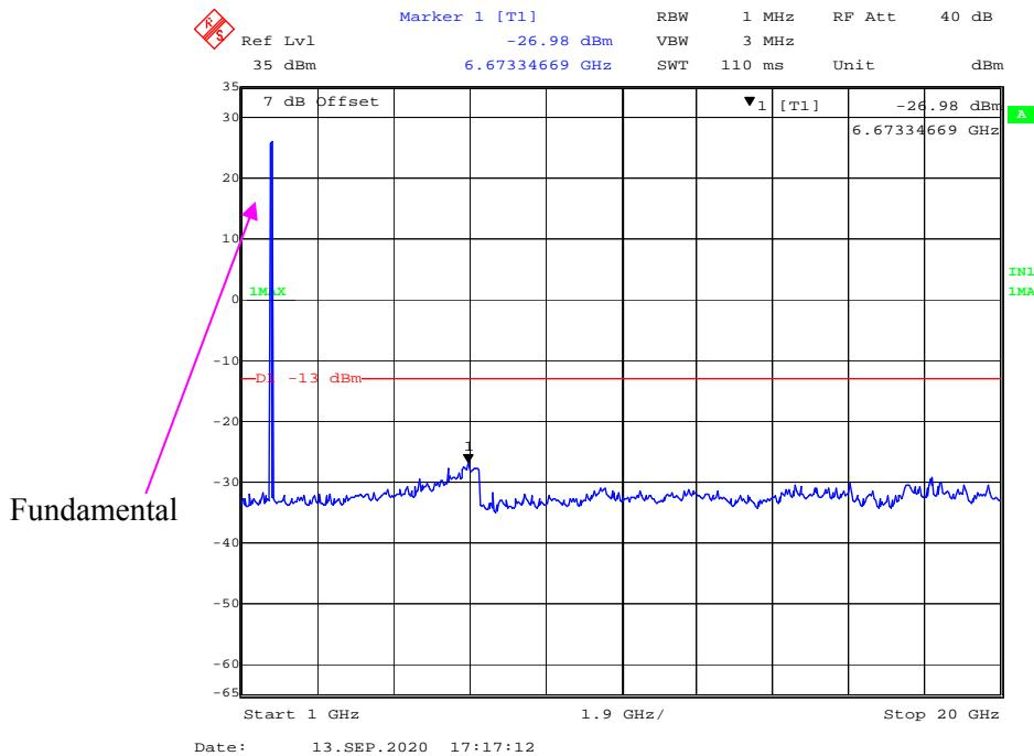
**LTE Band 2:****30 MHz - 1 GHz (1.4 MHz, QPSK, Low Channel)**
