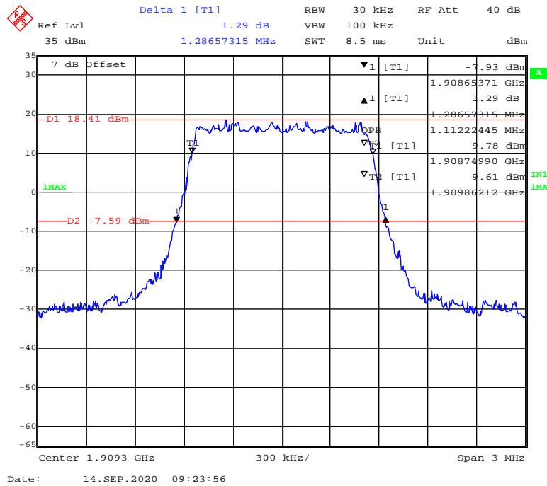
**16-QAM (3 MHz) - 99% Occupied & 26 dB Emissions Bandwidth, High channel**
