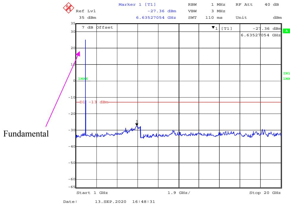
**WCDMA Band IV:****30 MHz – 1GHz WCDMA (Rel 99) Mode, Low channel**
