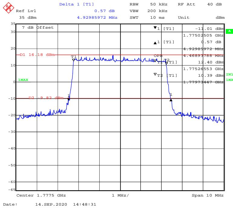
**QPSK (10MHz) - 99% Occupied & 26 dB Emissions Bandwidth, High channel**
