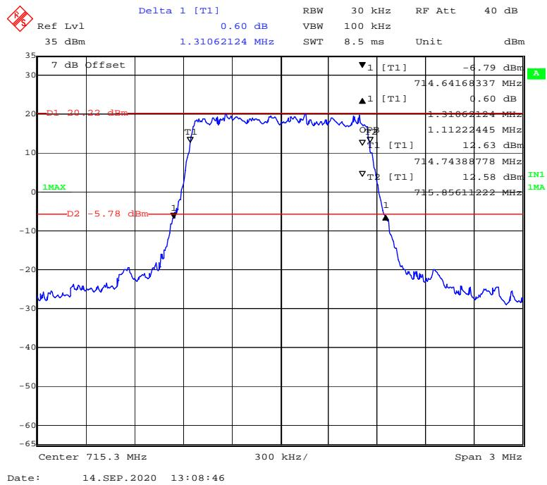
**QPSK (3 MHz) - 99% Occupied & 26 dB Emissions Bandwidth, High channel**
