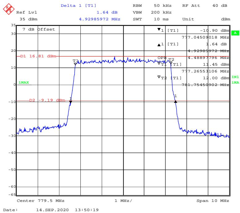
**QPSK (5 MHz) - 99% Occupied & 26 dB Emissions Bandwidth, Middle channel**
