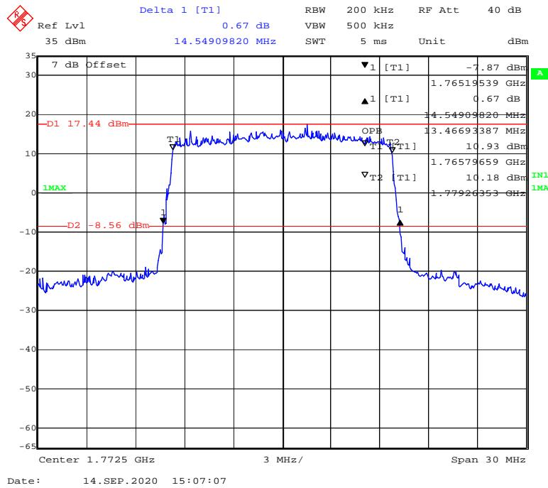
**16-QAM (20 MHz) - 99% Occupied & 26 dB Emissions Bandwidth, High channel**
