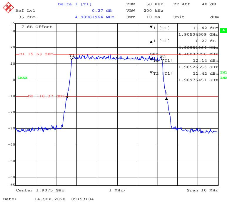
**16-QAM (10 MHz) - 99% Occupied & 26 dB Emissions Bandwidth, High channel**
