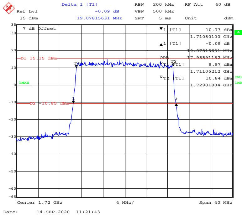
**16-QAM (1.4 MHz) - 99% Occupied & 26 dB Emissions Bandwidth, Low channel**
