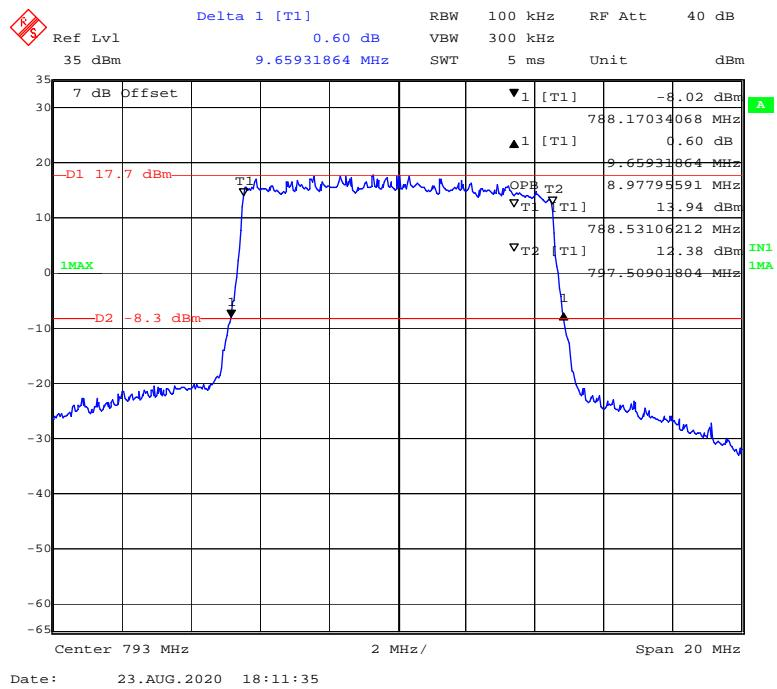
**16-QAM (5MHz) - 99% Occupied & 26 dB Emissions Bandwidth, Middle channel**
