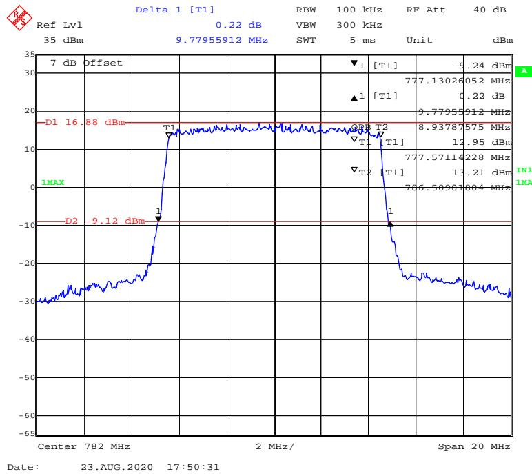
**QPSK (5 MHz) - 99% Occupied & 26 dB Emissions Bandwidth, High channel**
