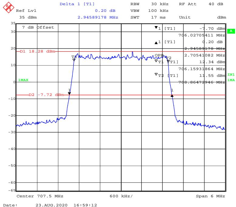
**QPSK (5 MHz) - 99% Occupied & 26 dB Emissions Bandwidth, Middle channel**
