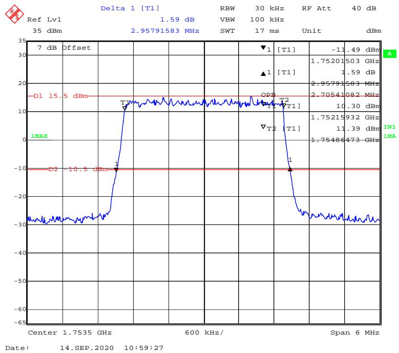
**QPSK (5MHz) - 99% Occupied & 26 dB Emissions Bandwidth, High channel**
