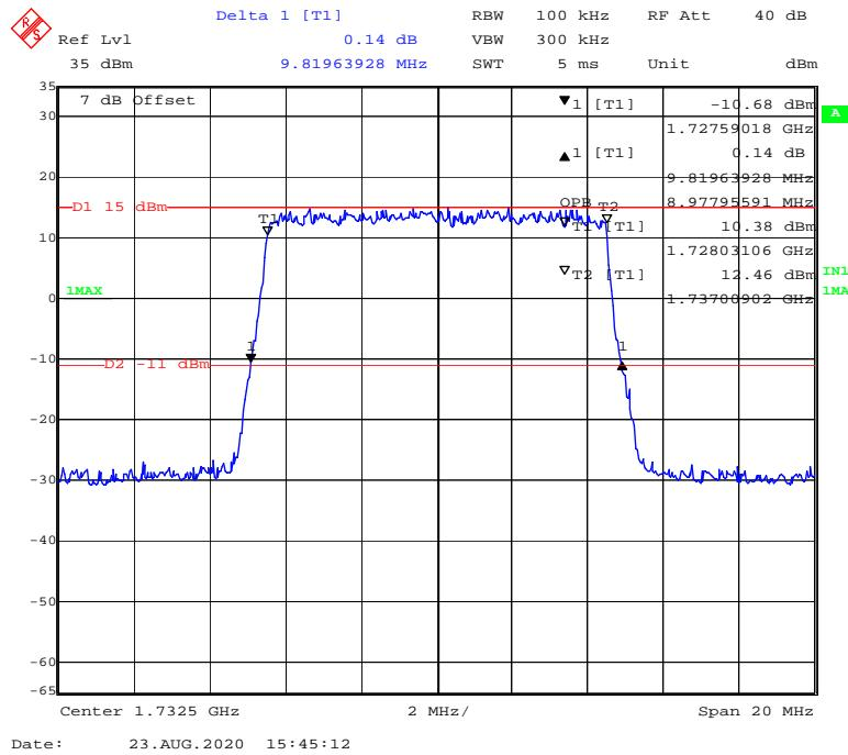
**16-QAM (15 MHz) - 99% Occupied & 26 dB Emissions Bandwidth, Middle channel**
