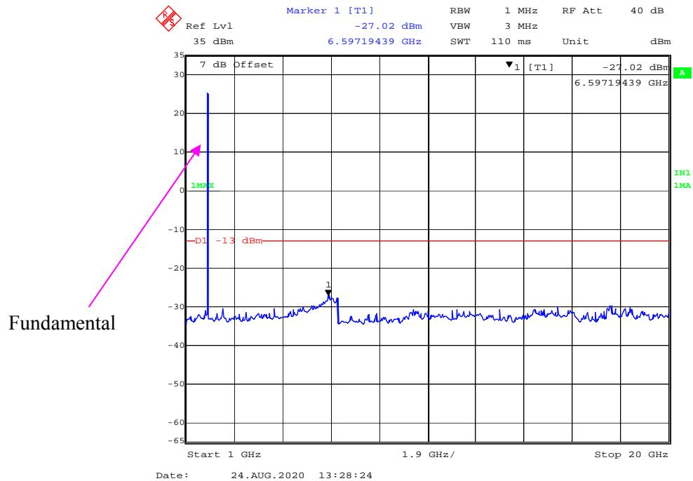
**30 MHz – 1GHz WCDMA (HSDPA) Mode, Middle channel**
