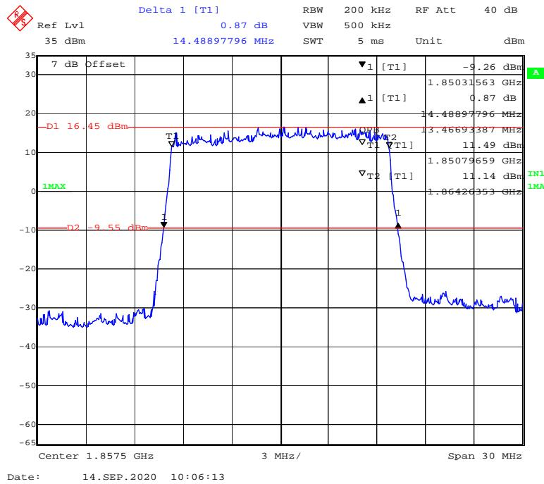
**16-QAM (20 MHz) - 99% Occupied & 26 dB Emissions Bandwidth, Low channel**
