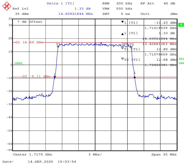
**QPSK (20 MHz) - 99% Occupied & 26 dB Emissions Bandwidth, Low channel**
