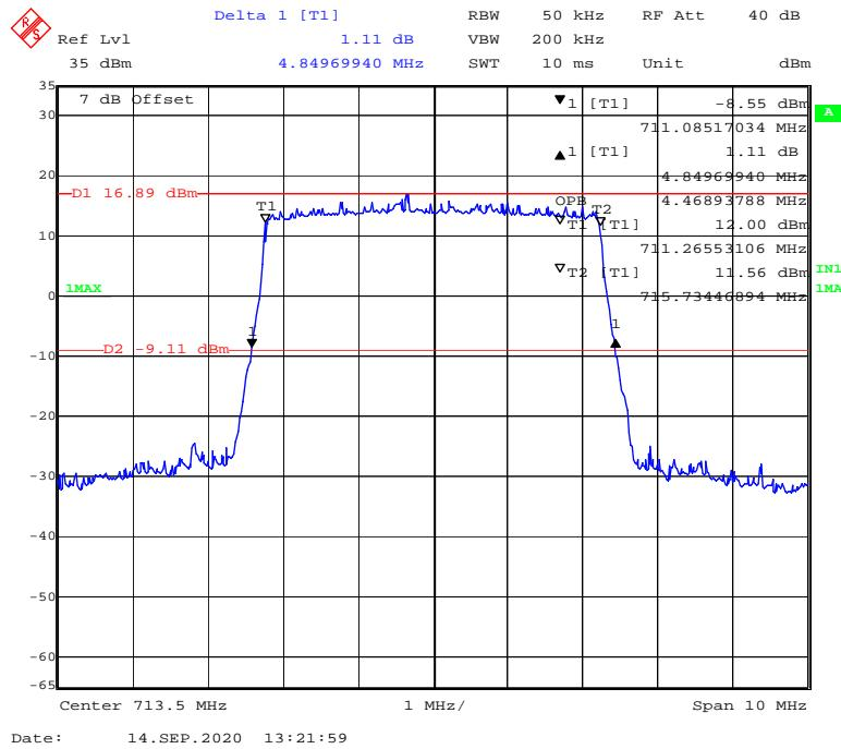
**QPSK (10MHz) - 99% Occupied & 26 dB Emissions Bandwidth, High channel**
