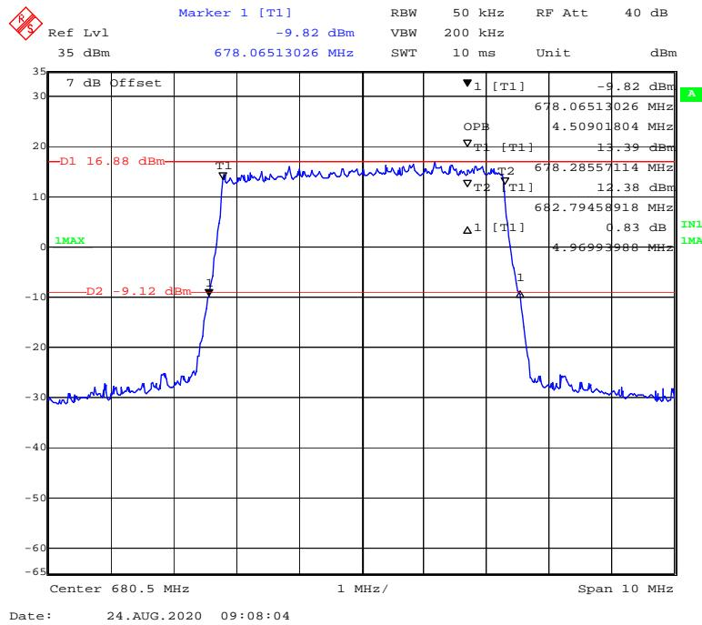
**QPSK (10MHz) - 99% Occupied & 26 dB Emissions Bandwidth, Middle channel**
