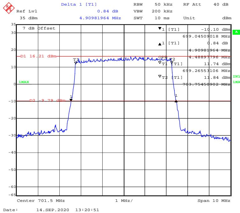
**16-QAM (10 MHz) - 99% Occupied & 26 dB Emissions Bandwidth, Low channel**
