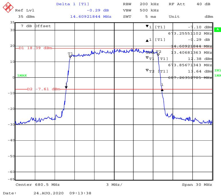
**QPSK (20 MHz) - 99% Occupied & 26 dB Emissions Bandwidth, Middle channel**
