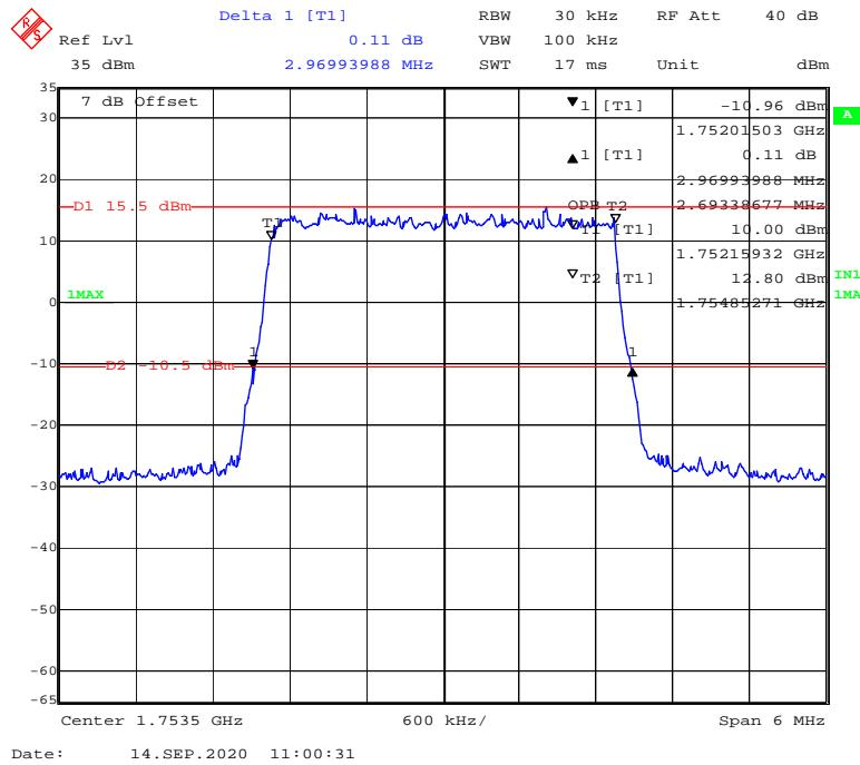
**16-QAM (5 MHz) - 99% Occupied & 26 dB Emissions Bandwidth, High channel**
