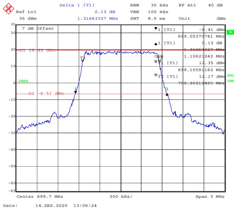
**QPSK (3 MHz) - 99% Occupied & 26 dB Emissions Bandwidth, Low channel**
