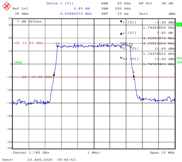
**QPSK (10MHz) - 99% Occupied & 26 dB Emissions Bandwidth, Middle channel**
