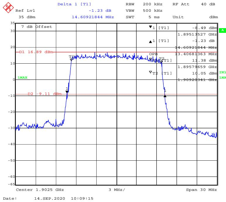
**16-QAM (20 MHz) - 99% Occupied & 26 dB Emissions Bandwidth, High channel**
