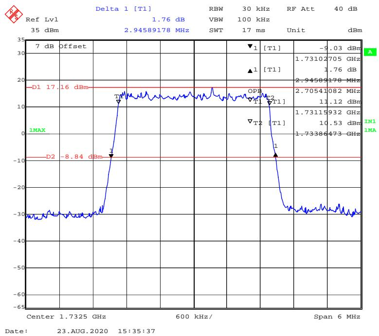
**QPSK (5MHz) - 99% Occupied & 26 dB Emissions Bandwidth, Middle channel**
