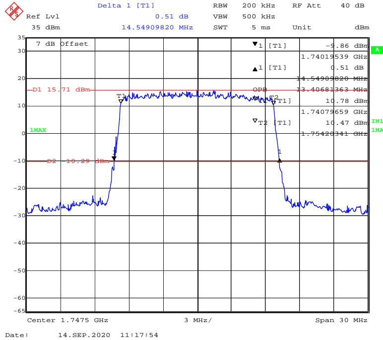
**16-QAM (20 MHz) - 99% Occupied & 26 dB Emissions Bandwidth, High channel**
