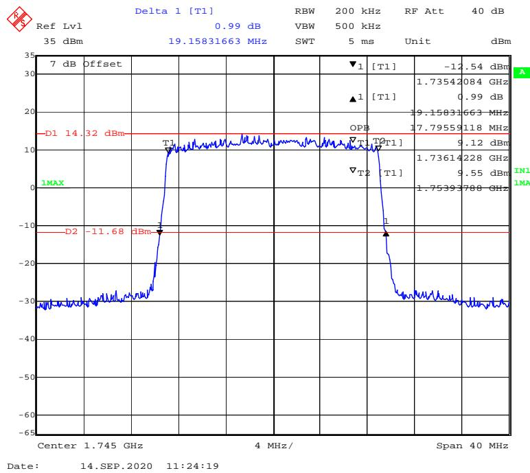
**16-QAM (1.4 MHz) - 99% Occupied & 26 dB Emissions Bandwidth, High channel**
