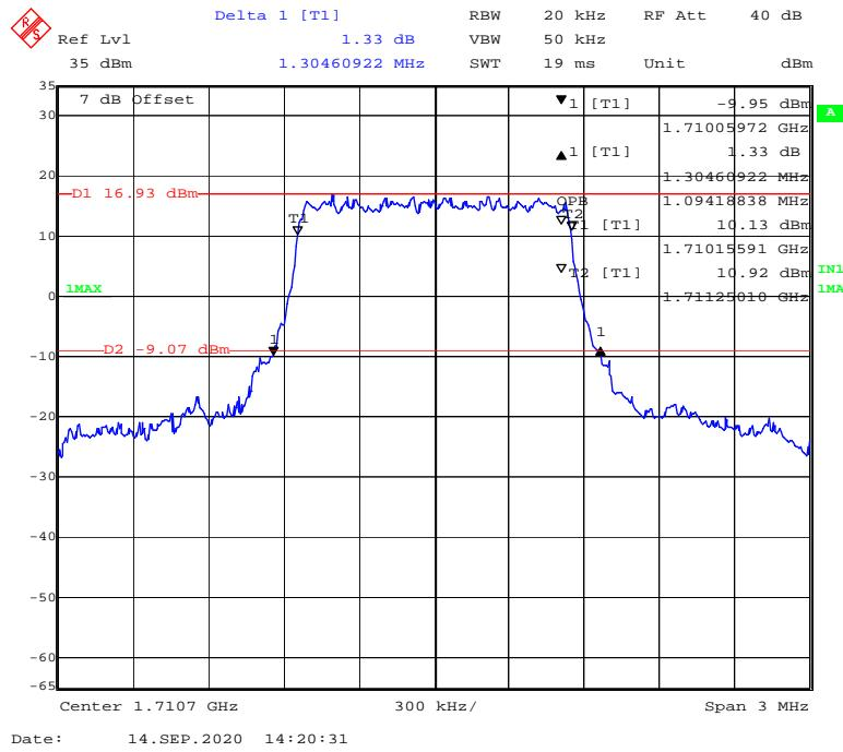
**16-QAM (3 MHz) - 99% Occupied & 26 dB Emissions Bandwidth, Low channel**
