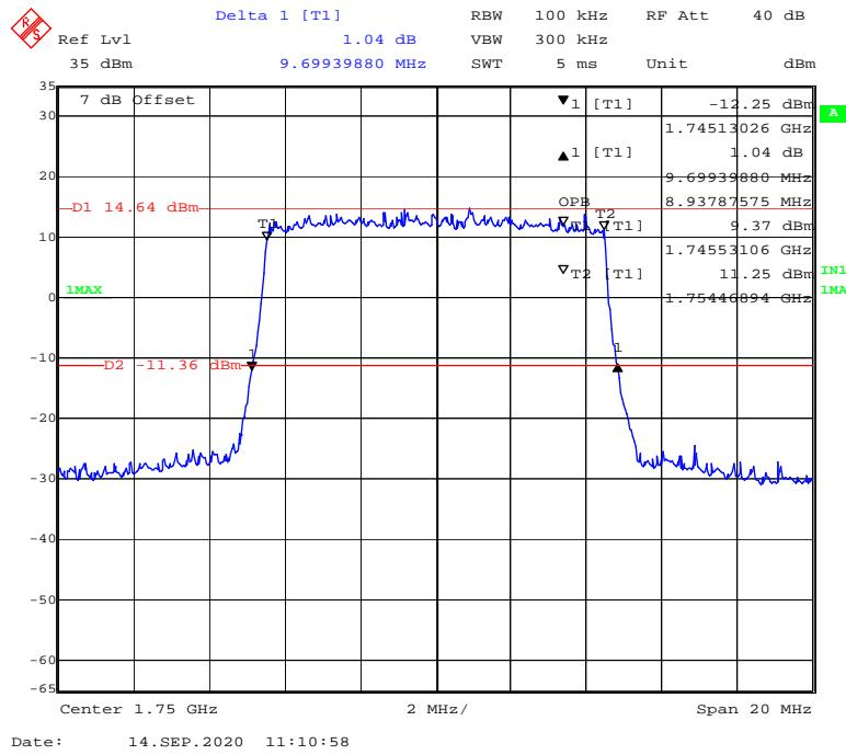
**16-QAM (15 MHz) - 99% Occupied & 26 dB Emissions Bandwidth, High channel**
