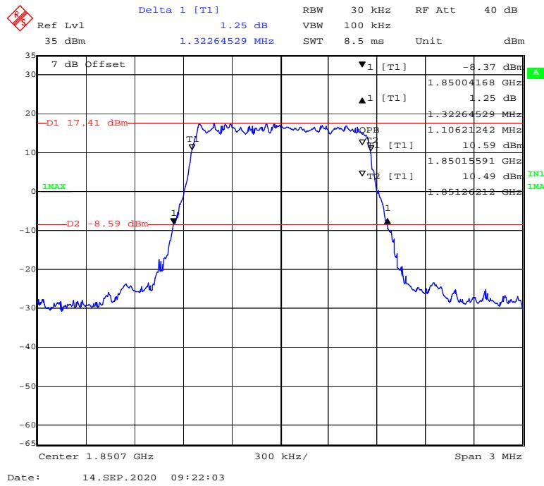
**16-QAM (3 MHz) - 99% Occupied & 26 dB Emissions Bandwidth, Low channel**
