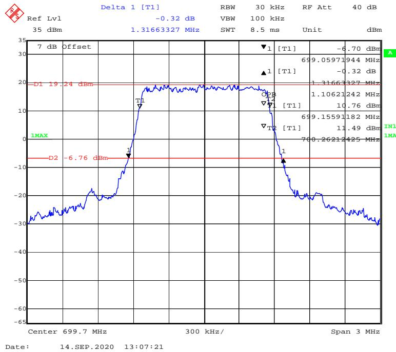
**16-QAM (3 MHz) - 99% Occupied & 26 dB Emissions Bandwidth, Low channel**
