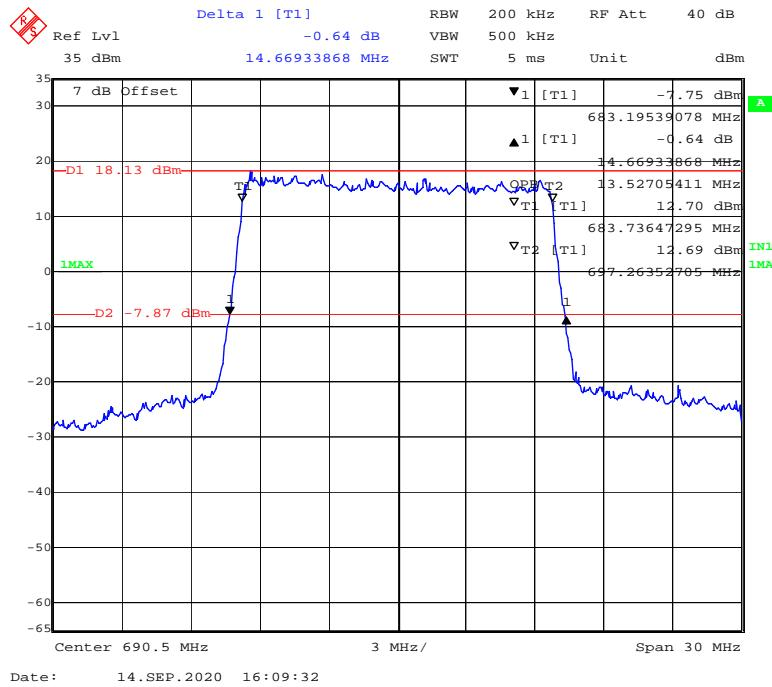
**QPSK (20 MHz) - 99% Occupied & 26 dB Emissions Bandwidth, High channel**
