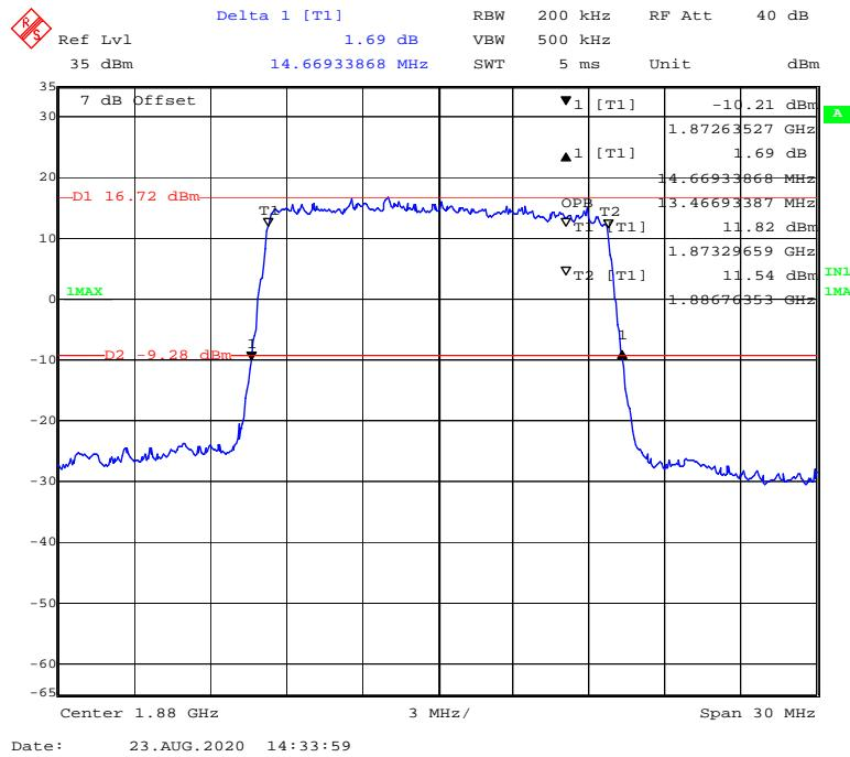
**16-QAM (20 MHz) - 99% Occupied & 26 dB Emissions Bandwidth, Middle channel**
