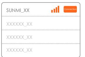
2. Open the browser, enter sunmi.link (or 192.168.100.1) in the address box to enter the quick configuration page and follow the prompts to complete the configuration.
