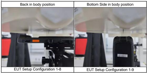
According to the antenna position and proximity ssensor status, the bbody SAR is tested at the following 1 test positions all with the distance =9mm between the EUT and the phantom bottom when the **sensor off**:
