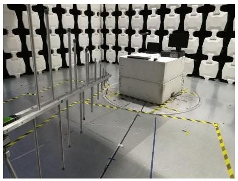
Description: Radiated Emission Test Setup
