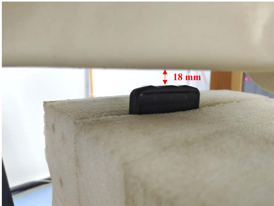
Body Bottom Setup Photo (Sensor off) (18mm)
