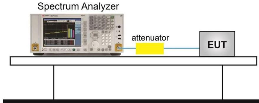
Note: The attenuator shown in the figure is the attenuation of the entire test system.
