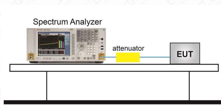
Note: The attenuator shown in the figure is the attenuation of the entire test system.
