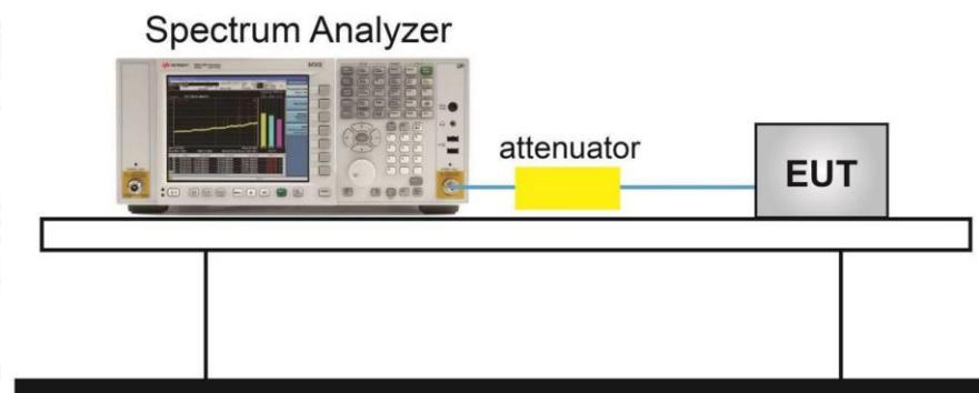
Note: The attenuator shown in the figure is the attenuation of the entire test system.
