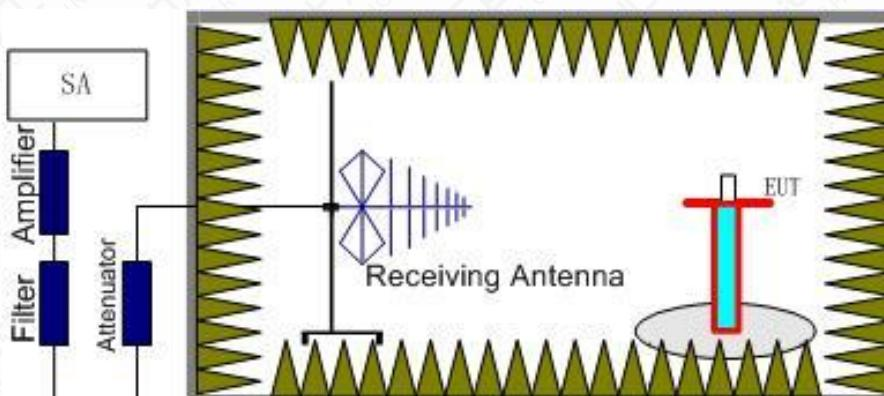
2.The EUT is then put into continuously transmitting mode at its maximum power level during the test.
