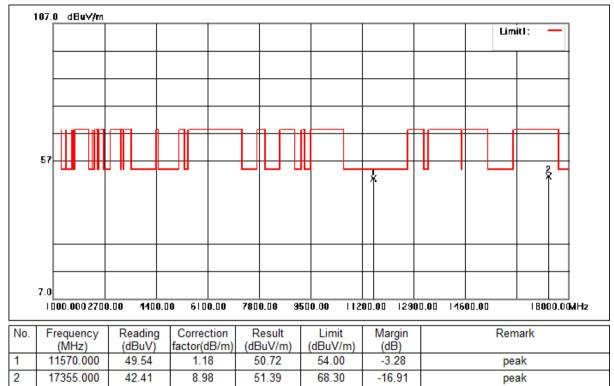
Mode:f; Polarization:Vertical; Modulation:a; bandwidth:20MHz; Channel:middle
