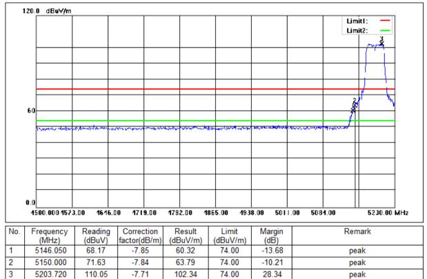
Mode:e; Polarization:Vertical; Modulation:n; bandwidth:40MHz; Channel:Low
