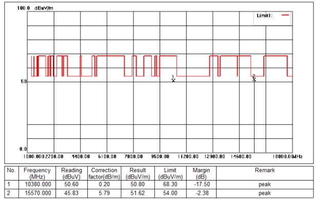
Mode:e; Polarization:Horizontal; Modulation:c; bandwidth:40MHz; Channel:Low
