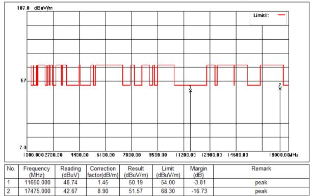
Mode:f; Polarization:Horizontal; Modulation:a; bandwidth:20MHz; Channel:High
