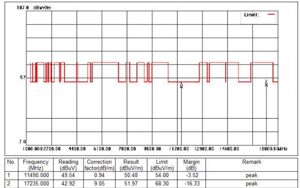
Mode:f; Polarization:Vertical; Modulation:n; bandwidth:20MHz; Channel:Low
