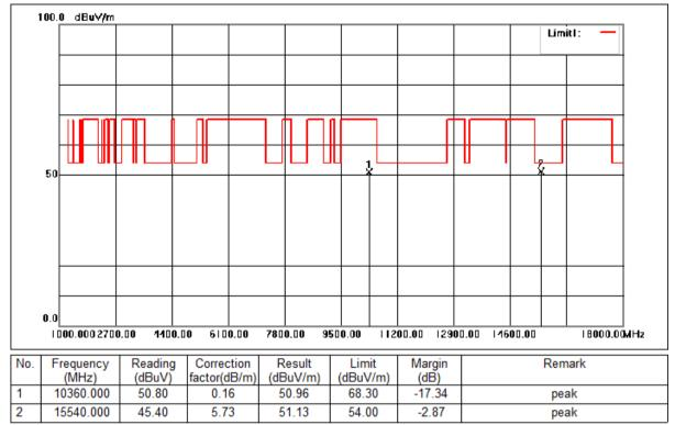
Mode:e; Polarization:Horizontal; Modulation:n; bandwidth:20MHz; Channel:Low
