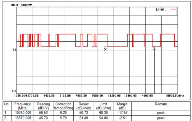
Mode:e; Polarization:Horizontal; Modulation:n; bandwidth:40MHz; Channel:Low
