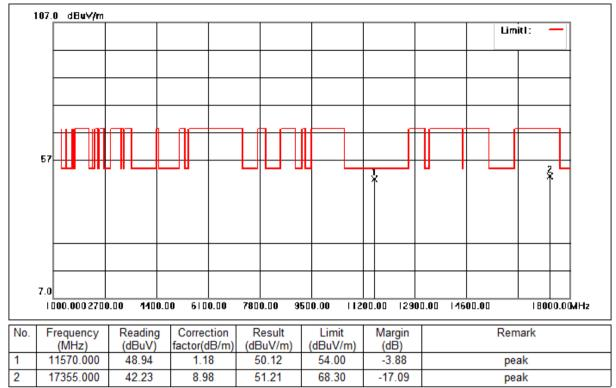
Mode:f; Polarization:Horizontal; Modulation:a; bandwidth:20MHz; Channel:middle
