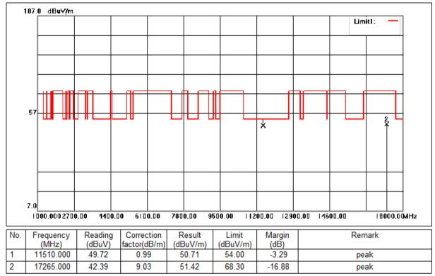
Mode:f; Polarization:Vertical; Modulation:c; bandwidth:40MHz; Channel:Low
