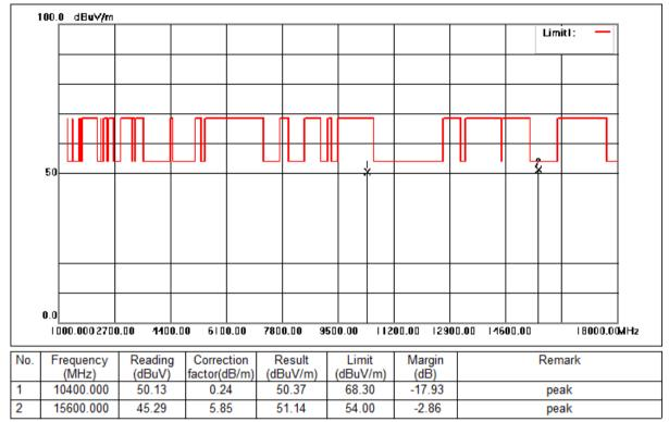
Mode:e; Polarization:Horizontal; Modulation:n; bandwidth:20MHz; Channel:middle
