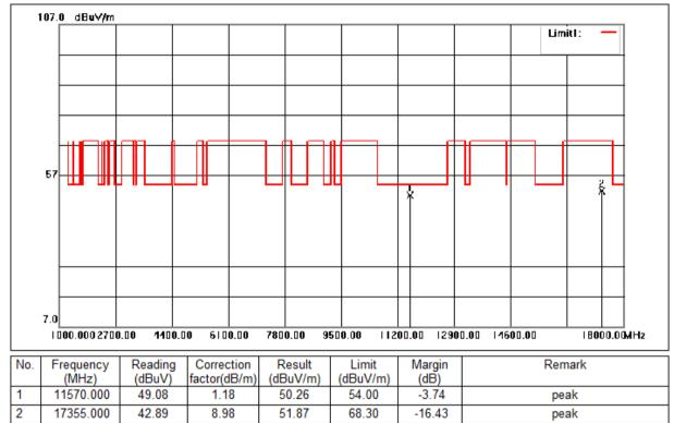
Mode:f; Polarization:Vertical; Modulation:c; bandwidth:20MHz; Channel:middle
