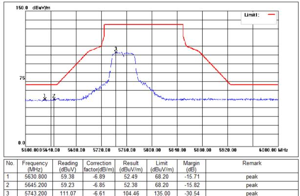
Mode:f; Polarization:Horizontal; Modulation:c; bandwidth:40MHz; Channel:Low
