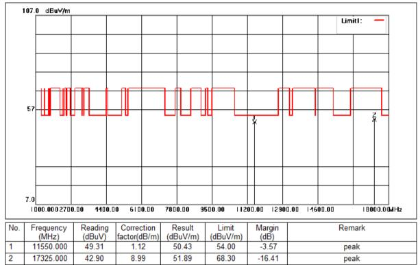
Mode:f; Polarization:Horizontal; Modulation:c; bandwidth:80MHz; Channel:middle
