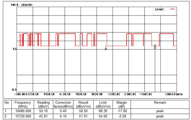
Mode:e; Polarization:Vertical; Modulation:c; bandwidth:20MHz; Channel:High
