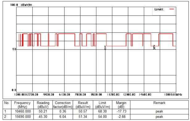
Mode:e; Polarization:Vertical; Modulation:c; bandwidth:40MHz; Channel:High
