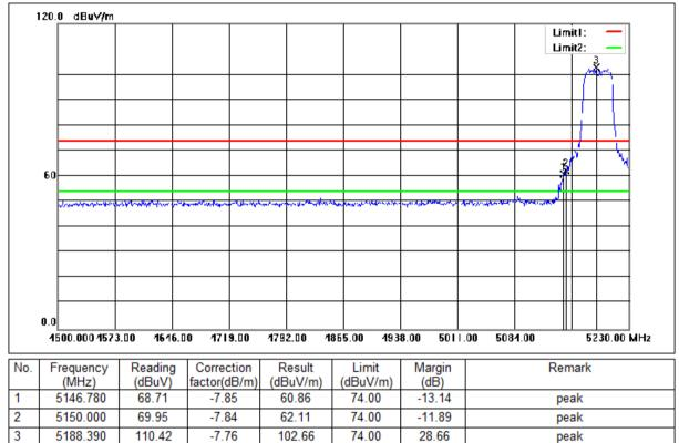
Mode:e; Polarization:Vertical; Modulation:c; bandwidth:40MHz; Channel:Low
