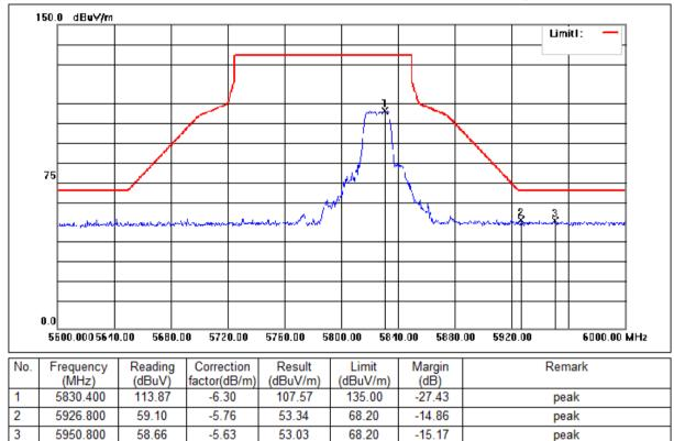
Mode:f; Polarization:Horizontal; Modulation:c; bandwidth:20MHz; Channel:High
