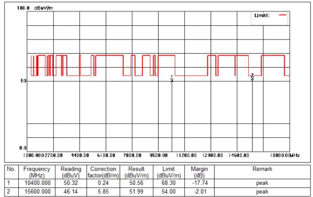
Mode:e; Polarization:Horizontal; Modulation:c; bandwidth:20MHz; Channel:middle
