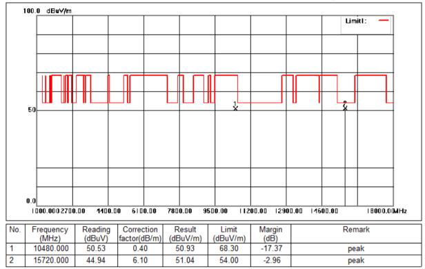
Mode:e; Polarization:Horizontal; Modulation:c; bandwidth:20MHz; Channel:High
