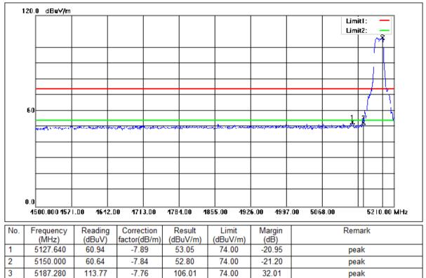
Mode:e; Polarization:Vertical; Modulation:a; bandwidth:20MHz; Channel:Low
