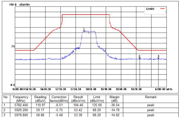
Mode:f; Polarization:Vertical; Modulation:n; bandwidth:40MHz; Channel:High
