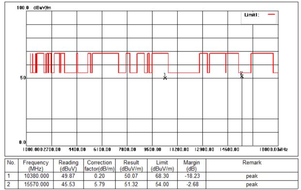
Mode:e; Polarization:Vertical; Modulation:c; bandwidth:40MHz; Channel:Low
