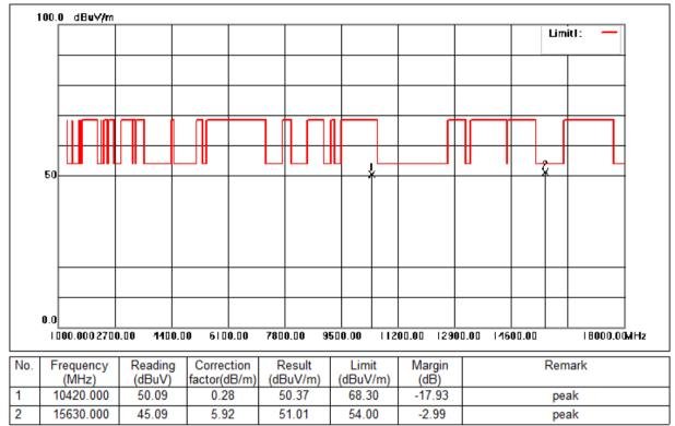
Mode:e; Polarization:Horizontal; Modulation:c; bandwidth:80MHz; Channel:middle
