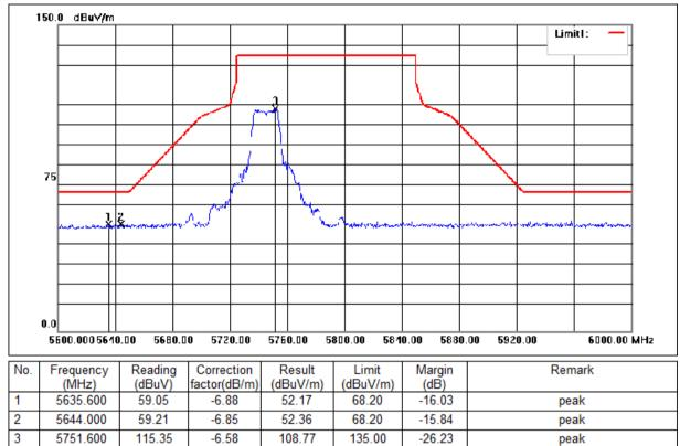
Mode:f; Polarization:Vertical; Modulation:c; bandwidth:20MHz; Channel:Low
