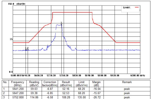
Mode:f; Polarization:Horizontal; Modulation:c; bandwidth:20MHz; Channel:Low
