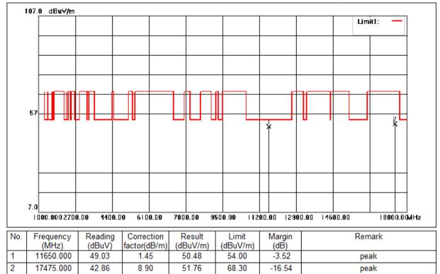
Mode:f; Polarization:Horizontal; Modulation:c; bandwidth:20MHz; Channel:High
