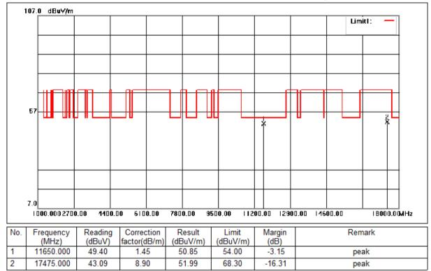
Mode:f; Polarization:Vertical; Modulation:n; bandwidth:20MHz; Channel:High
