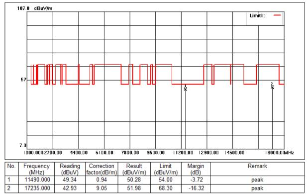
Mode:f; Polarization:Vertical; Modulation:a; bandwidth:20MHz; Channel:Low
