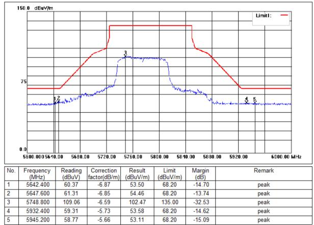
Mode:f; Polarization:Horizontal; Modulation:c; bandwidth:80MHz; Channel:Low
