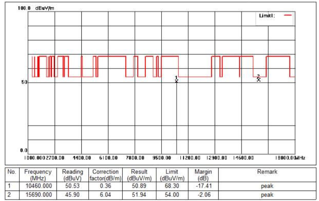
Mode:e; Polarization:Horizontal; Modulation:c; bandwidth:40MHz; Channel:High
