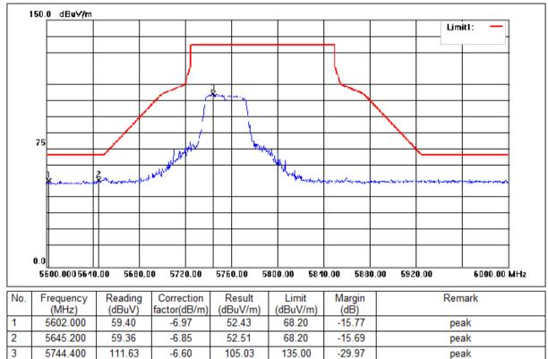
Mode:f; Polarization:Vertical; Modulation:n; bandwidth:40MHz; Channel:Low
