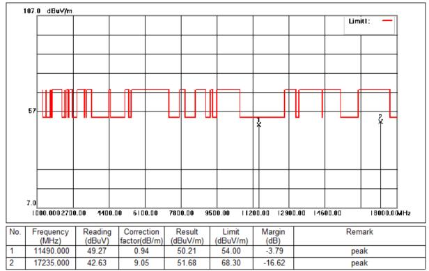
Mode:f; Polarization:Horizontal; Modulation:c; bandwidth:20MHz; Channel:Low
