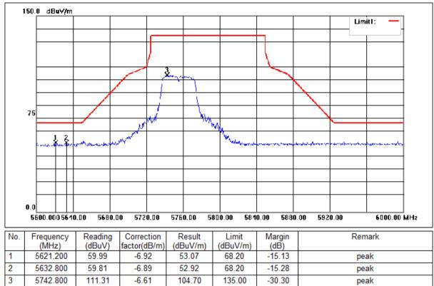
Mode:f; Polarization:Horizontal; Modulation:n; bandwidth:40MHz; Channel:Low
