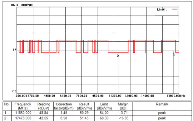
Mode:f; Polarization:Vertical; Modulation:c; bandwidth:20MHz; Channel:High
