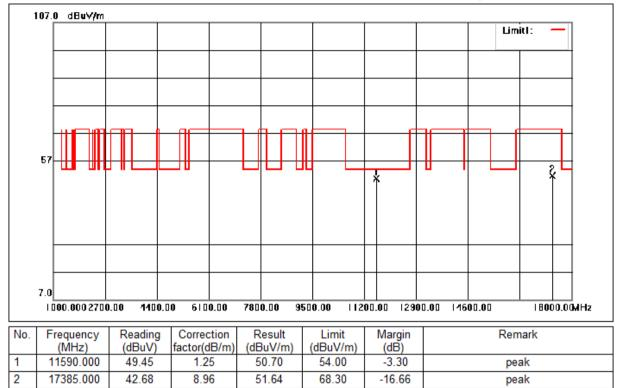
Mode:f; Polarization:Horizontal; Modulation:n; bandwidth:40MHz; Channel:High
