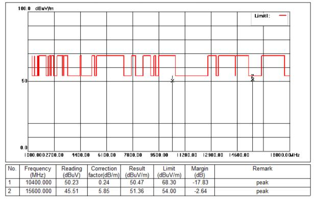
Mode:e; Polarization:Vertical; Modulation:n; bandwidth:20MHz; Channel:middle
