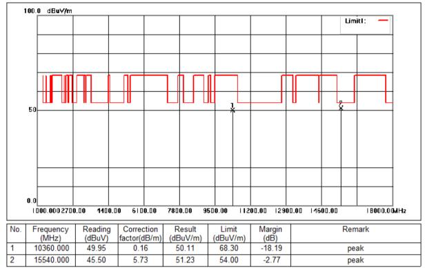
Mode:e; Polarization:Vertical; Modulation:c; bandwidth:20MHz; Channel:Low
