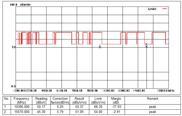
Mode:e; Polarization:Vertical; Modulation:n; bandwidth:40MHz; Channel:Low
