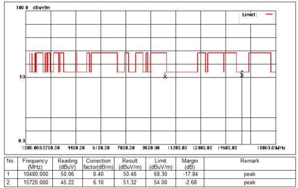
Mode:e; Polarization:Horizontal; Modulation:a; bandwidth:20MHz; Channel:High
