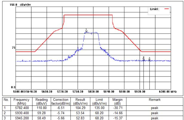
Mode:f; Polarization:Horizontal; Modulation:n; bandwidth:40MHz; Channel:High
