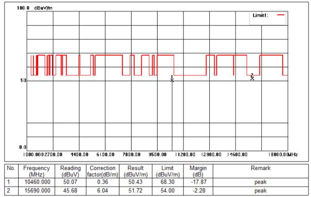
Mode:e; Polarization:Horizontal; Modulation:n; bandwidth:40MHz; Channel:High
