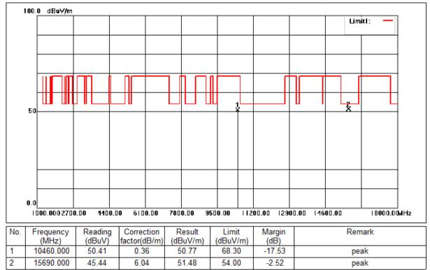
Mode:e; Polarization:Vertical; Modulation:n; bandwidth:40MHz; Channel:High
