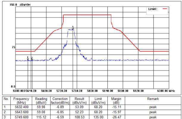
Mode:f; Polarization:Vertical; Modulation:a; bandwidth:20MHz; Channel:Low
