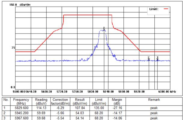
Mode:f; Polarization:Horizontal; Modulation:a; bandwidth:20MHz; Channel:High
