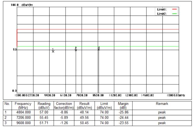
Mode:c; Polarization:Vertical; Modulation:GFSK; ; Channel:Low
