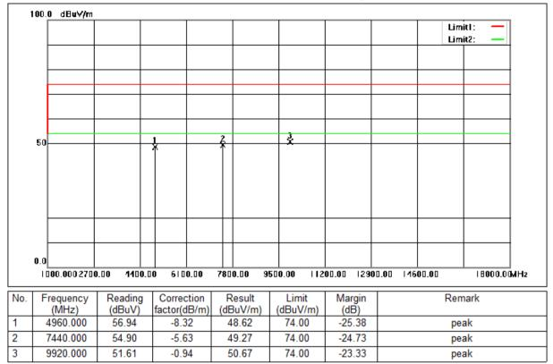
Mode:c; Polarization:Horizontal; Modulation:GFSK; ; Channel:High
