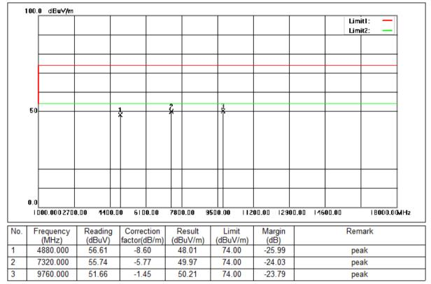
Mode:c; Polarization:Horizontal; Modulation:GFSK; ; Channel:middle
