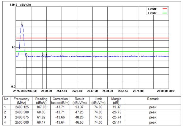
Mode:c; Polarization:Horizontal; Modulation:GFSK; ; Channel:High
