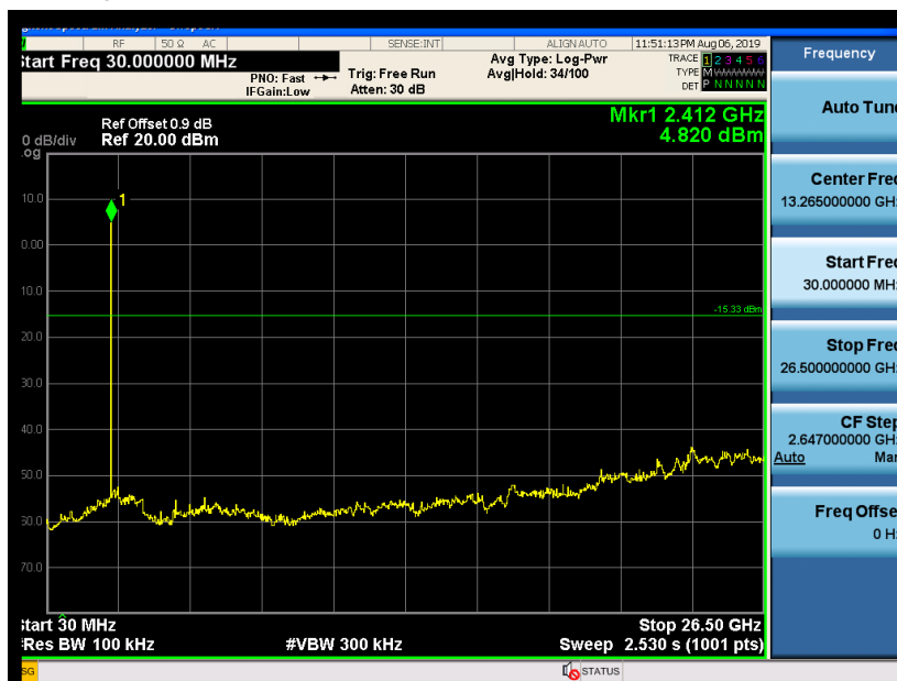
Fig.13 Conducted spurious emission: Ch0, 30MHz~26GHz
