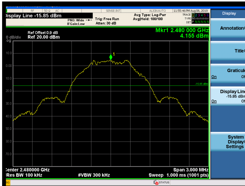
Fig.16 Conducted spurious emission: Ch39, 2480MHz
