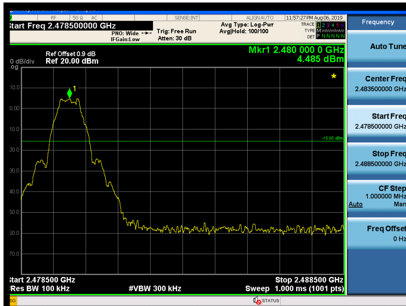
Fig.11 Frequency Band Edge: GFSK, Ch39
