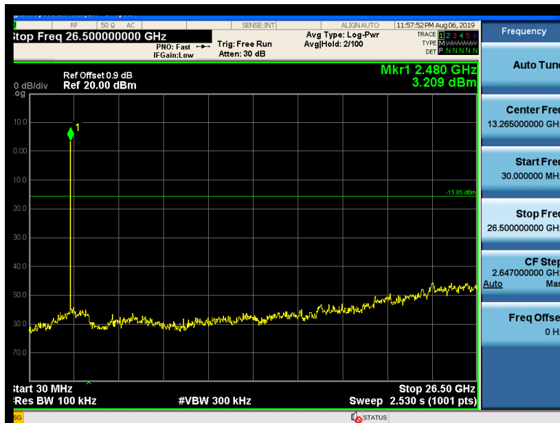
Fig.17 Conducted spurious emission: Ch39, 30MHz~26GHz
