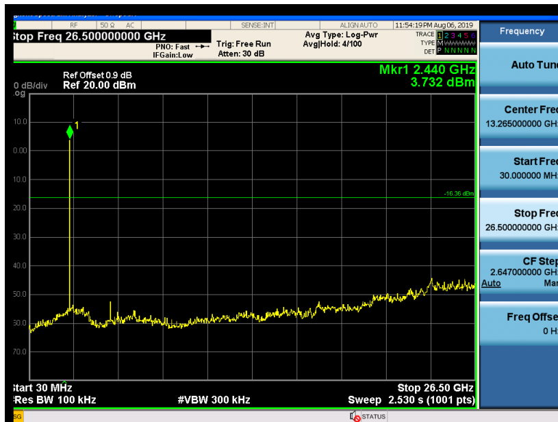
Fig.15 Conducted spurious emission: Ch19, 30MHz~26GHz
