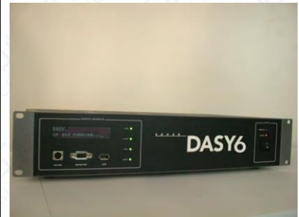
Figure 7.4.3-1 Server for DASY6
