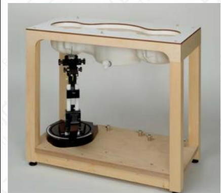
Figure 7.4.5-1: SAM Twin Phantom
