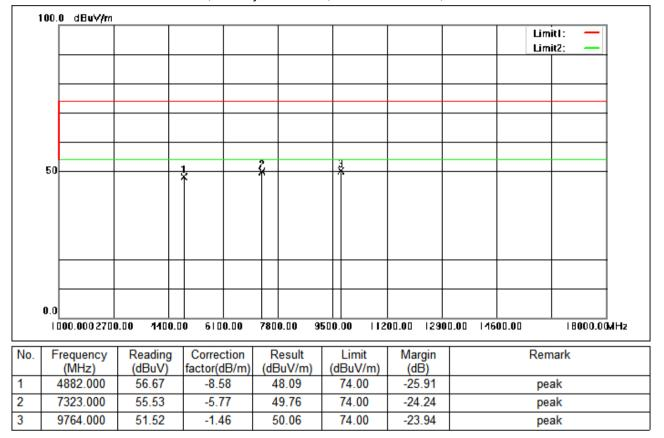
Test Mode: 01; Polarity: Horizontal; Modulation:GFSK; Channel:middle
