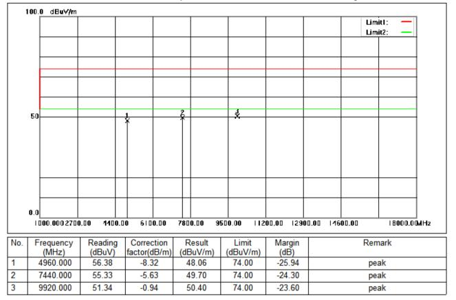
Test Mode: 01; Polarity: Vertical; Modulation:8DPSK; Channel:High
