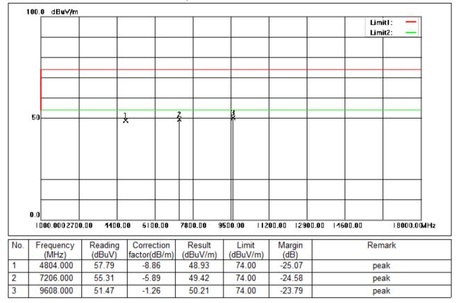
Test Mode: 01; Polarity: Vertical; Modulation:GFSK; Channel:Low
