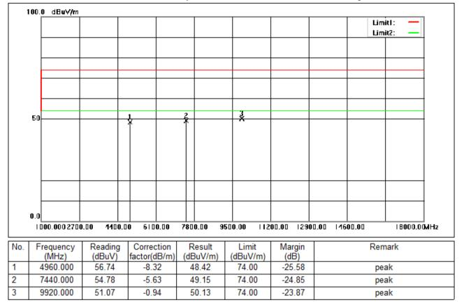
Test Mode: 01; Polarity: Vertical; Modulation:GFSK; Channel:High
