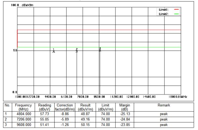
Test Mode: 01; Polarity: Vertical; Modulation:GFSK; Channel:Low
