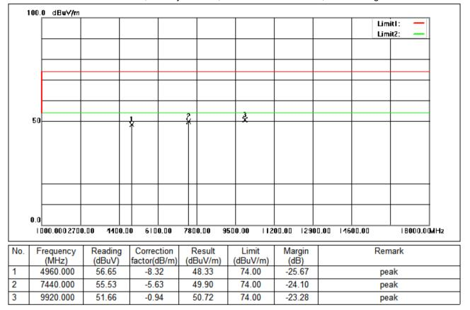
Test Mode: 01; Polarity: Vertical; Modulation:π/4 DQPSK; Channel:High
