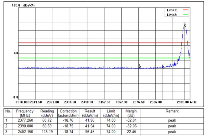
Test Mode: 01; Polarity: Vertical; Modulation:GFSK; Channel:Low
