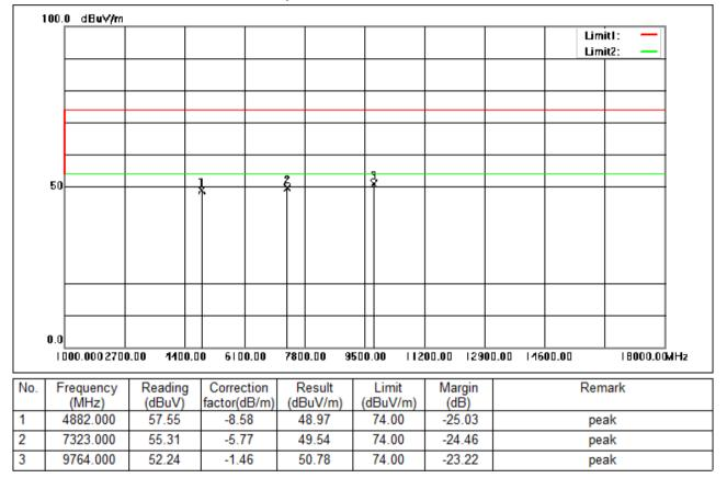
Test Mode: 01; Polarity: Vertical; Modulation:GFSK; Channel:middle
