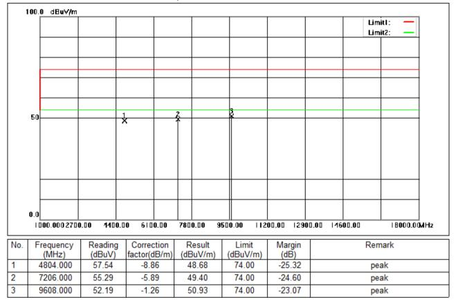
Test Mode: 01; Polarity: Horizontal; Modulation:8DPSK; Channel:Low
