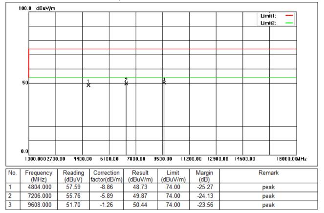
Test Mode: 01; Polarity: Horizontal; Modulation:π/4 DQPSK; Channel:Low
