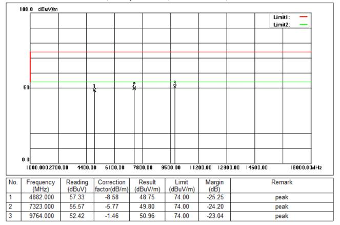
Test Mode: 01; Polarity: Horizontal; Modulation:GFSK; Channel:middle
