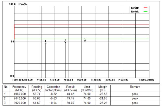
Test Mode: 01; Polarity: Vertical; Modulation:8DPSK; Channel:High
